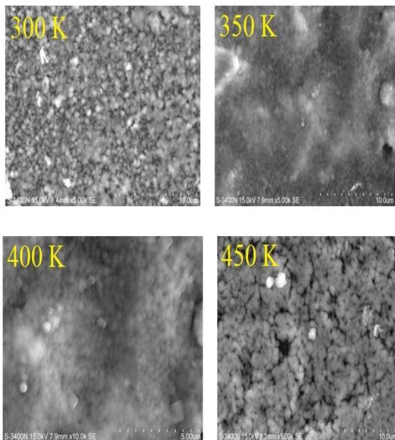
**Figure 4b:** SEM image of AIO thin film as a function of different substrate temperature.
