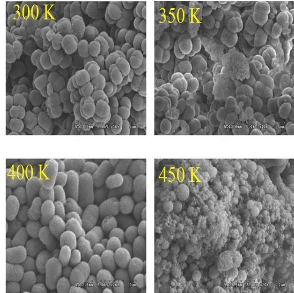
**Figure 4a:** SEM image of CIO thin film as a function of different substrate temperature.
