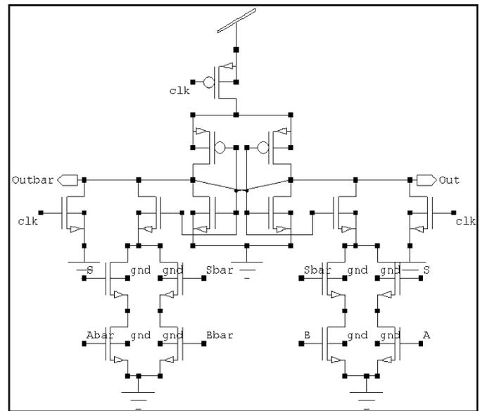
Fig. 6. Schematic of DCSL2 circuit
