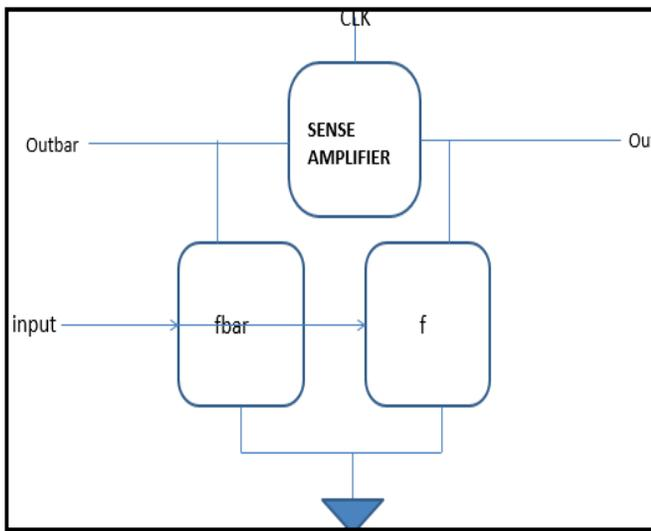
Fig. 1. Circuit arrangement for simulation of sense-amplifier circuits
