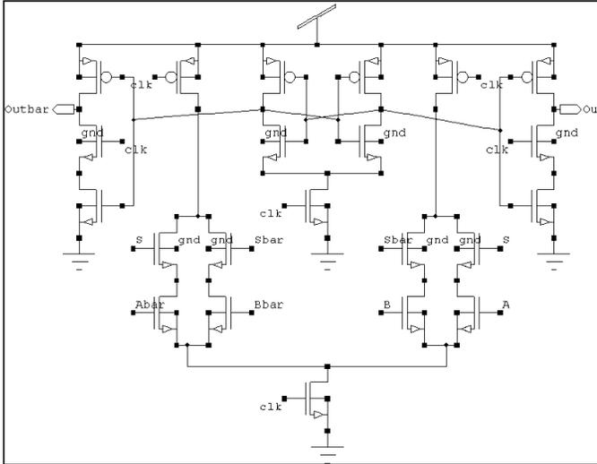
Fig. 4. Schematic of LCDL circuit
