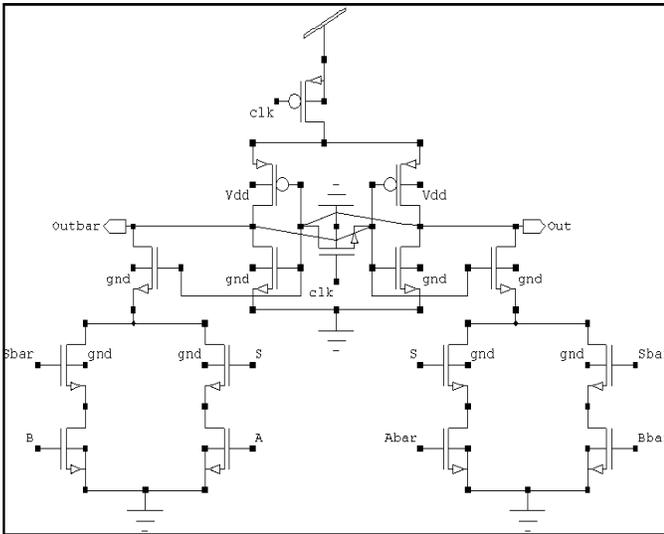
Fig. 7. Schematic of DC SL3 circuit
