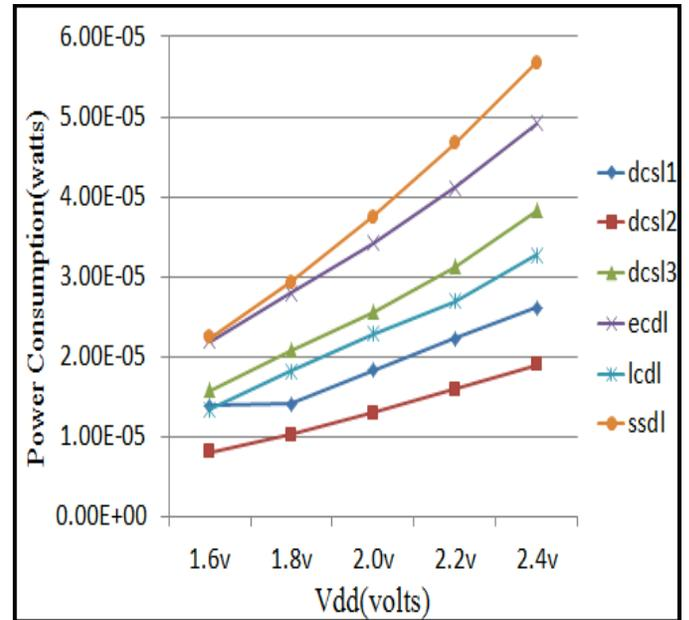
Fig. 8. Power Consumption vs Vdd for dcs11, dcs12, dcs13, ecd1, lcd1, ssd1 based Multiplexers circuits.
