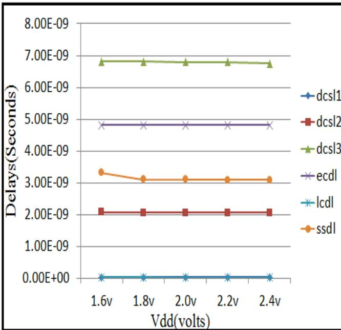
Fig. 11. Delay vs Vdd for dcs1, dcs2, dcs3, ecdl, lcdl, ssdl based Multiplexer circuit.
