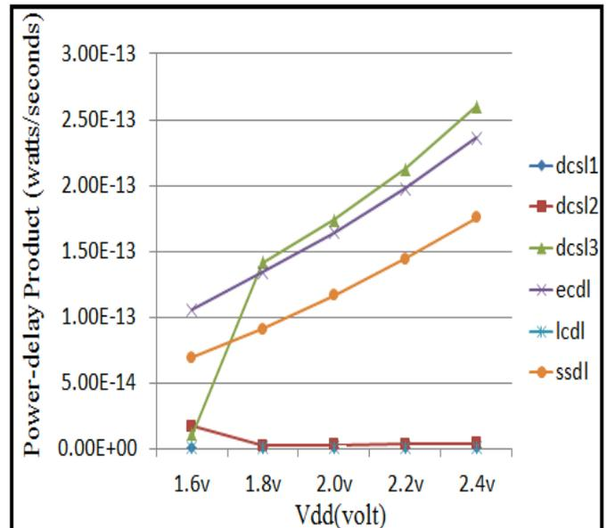
Fig. 12. Power delay product vs Vdd for dcs1, dcs2, dcs3, ecdl, lcdl, ssdl of 2:1 Multiplex circuit.
