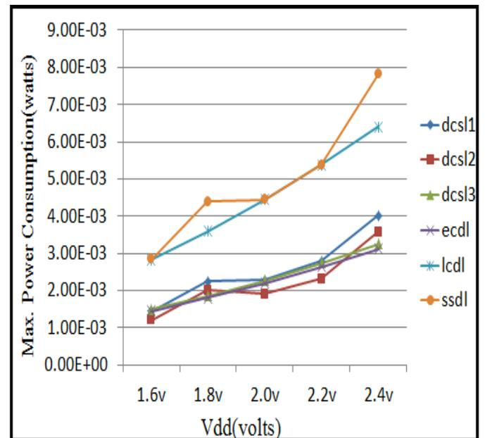
Fig. 9. Maximum Power Consumption vs Vdd for dcs11, dcs12, dcs13, ecd1, lcd1, ssd1 based Multiplexers circuits.
