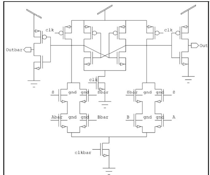
Fig. 2. Schematic of SSDL circuit
