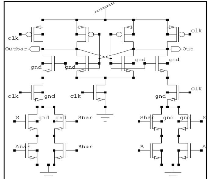
Fig. 5. Schematic of DCSL1 circuit
