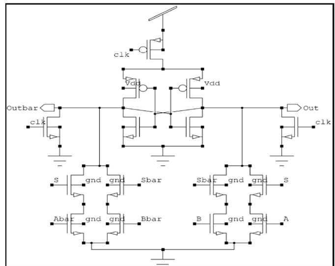
Fig. 3. Schematic of ECDL circuit
