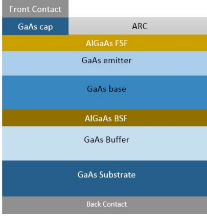
Fig. 1. Cross Section of simulated GaAs solar cell. (Figure not to scale)
