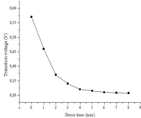
**Figure 4:** The transition voltage of the emitter–base junction of a standard bipolar transistor as a function of the stress duration (reverse junction bias).
