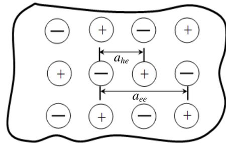
**Figure 2** Average geometrical order of electrons and holes in highly excited intrinsic semiconductors.
