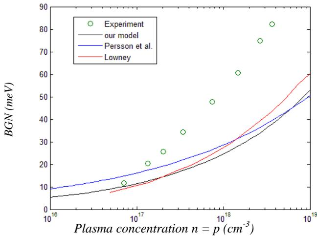
**Figure 4** Comparison of rigid BGN between our model, Persson *et al.*, and Lowney models, along with the experimental data by Neugroschel *et al.*
