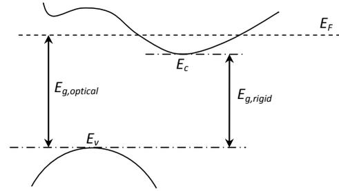
**Figure 1** The difference between the rigid and optical band gap energy for n-type doping silicon.
