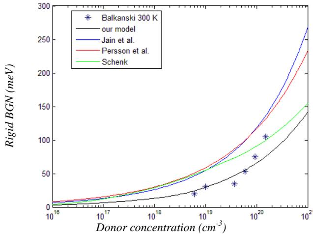
**Figure 6** Comparison of rigid BGN models with experimental data for n-type Si at  $T = 300$  K.
