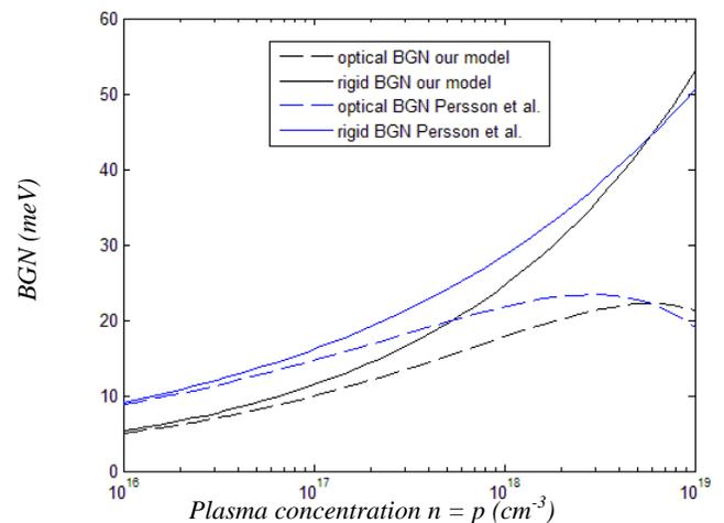
**Figure 3** Comparison of rigid and optical BGN between our model and the model by Persson *et al.*
