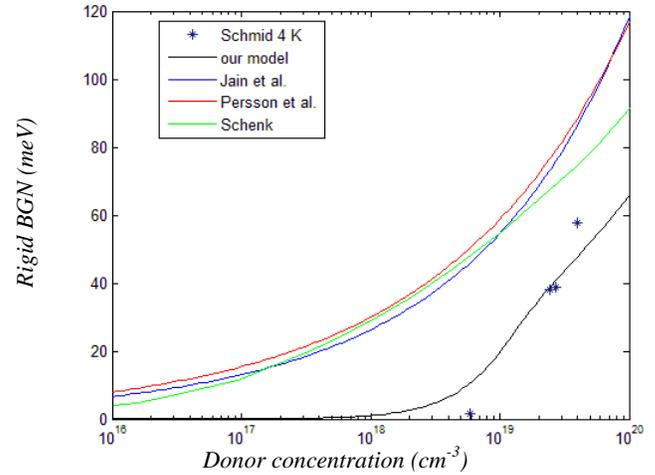
**Figure 7** Comparison of rigid BGN models with experimental data for n-type Si at  $T = 4$  K.
