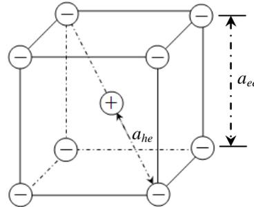
**Figure 5** Electrons and holes average distribution in n-type semiconductor.
