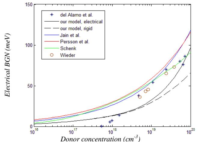
**Figure 8** Comparison of electrical BGN from experiments and theoretical models with our model.
