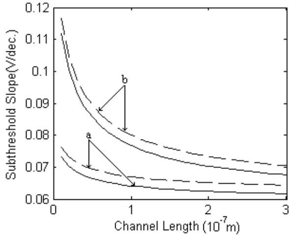
Fig. 5. Plot of Subthreshold slope with channel length for SOI (dashed line) and SON (solid line) MOSFET. Parameter values are same as in Fig.1 and also the symbols have the same significance.
