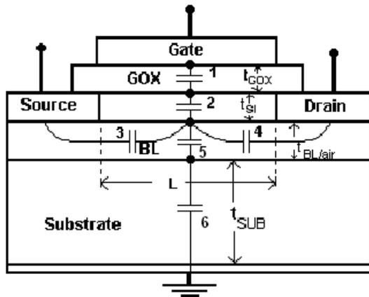
Fig. 1. A SOI/SON-MOSFET layered structure.
