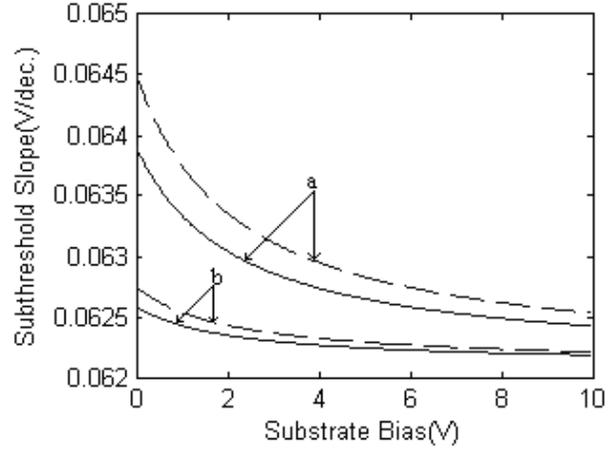
Fig. 11. Subthreshold slope with substrate bias for SON (dashed line) and SOI (solid line) MOSFET. Significance of symbol and parameters values is same as in Fig.6.
