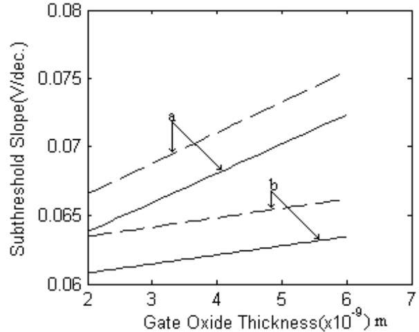
Fig. 7. Subthreshold Slope with gate oxide thickness for SOI (dashed line) and SON (solid line) MOSFET. Significance of symbol and parameters values is same as in Fig.6.
