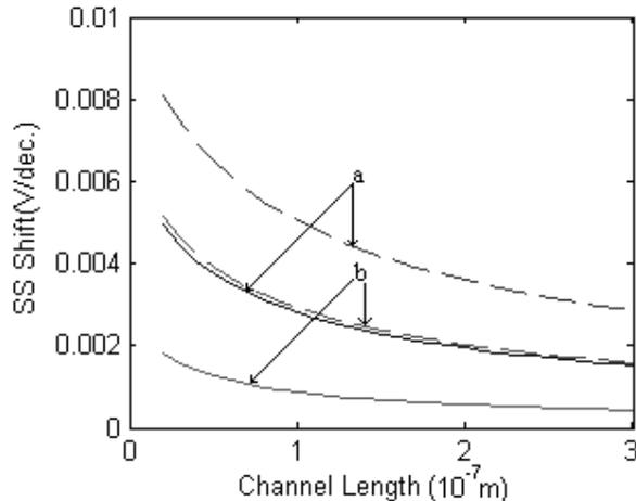
Fig. 10. Subthreshold slope (SS) shift with channel length for SON (dashed line) and SOI (solid line) MOSFET. Significance of symbol and parameters values is same as in Fig.6.
