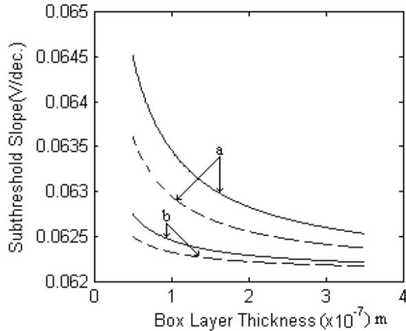
Fig. 9. Subthreshold slope with gate oxide thickness for SON (dashed line) and SOI (solid line) MOSFET. Significance of symbol and parameters values is same as in Fig.6.
