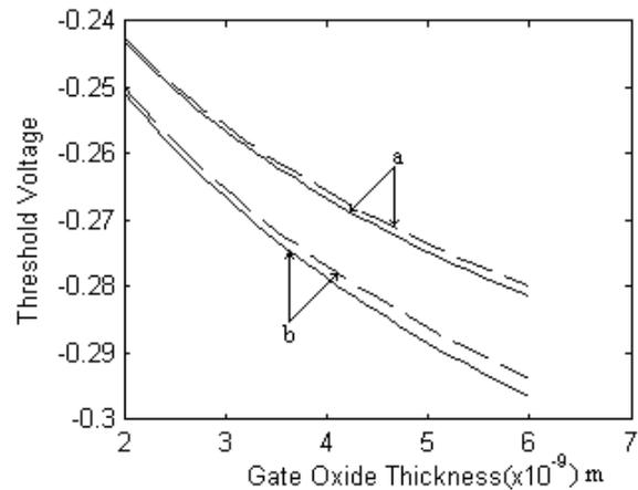
Fig. 6. Threshold voltage with gate oxide thickness for SON (dashed line) and SOI (solid line) MOSFET. Back-gate voltage  $V_B = 0$  V,  $V_{DS} = 1$  V,  $T_{BOX}=147$ nm,  $N_a=0.5 \cdot 10^{14}$  cm<sup>-2</sup>,  $N_{sub}=4 \cdot 10^{12}$  cm<sup>-2</sup>,  $L=50$ nm. Curve a:  $V_{DS} = 1$  V and curve b:  $V_{DS} = 0.05$  V. Other parameters are same as in Fig. 1.
