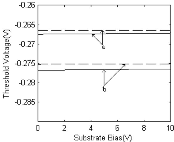
Fig. 10. Threshold voltage with substrate bias for SON (dashed line) and SOI (solid line) MOSFET. Significance of symbol and parameters values is same as in Fig.6.
