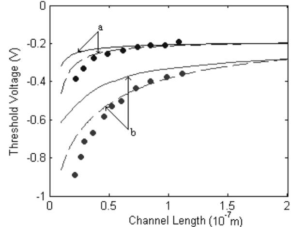
Fig. 4. Plot of Threshold voltage with channel length for SOI (dashed line) and SON (solid line) MOSFET. Back-gate voltage  $V_B = 0$  V,  $V_{DS} = 1$  V,  $T_{GOX}=5$ nm,  $T_{BOX}=147$ nm,  $N_a=0.5 \cdot 10^{14}$  cm<sup>-2</sup>,  $N_{sub}=4 \cdot 10^{12}$  cm<sup>-2</sup>. Curve a:  $T_{Si} = 8.6$  and curve b:  $T_{Si} = 18.2$
