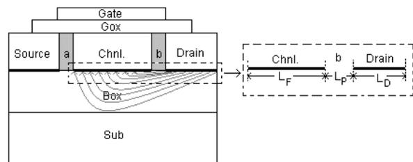
Fig: 3. Fringing capacitance model of SOI/SON-MOSFET.
