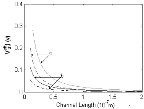
Fig. 12.  $|V_{th}^{sft}|$  with channel length for SON (dashed line) and SOI (solid line) MOSFET. Significance of symbol and parameters values is same as in Fig.6.
