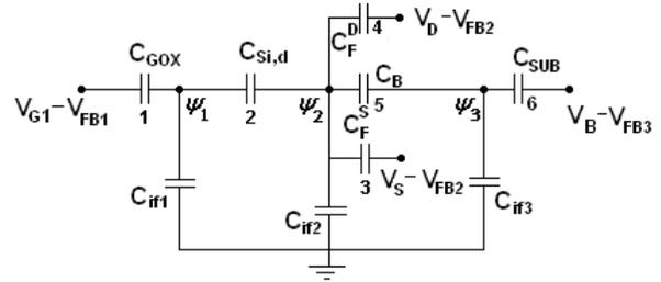
Fig. 2. Equivalent capacitance model of SOI/SON-MOSFET
