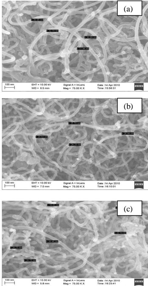
**FIGURE 3.** FESEM images of CNTs with different diameter on (a)  $Mg_{0.1}Zn_{0.9}O$ ; (b)  $Mg_{0.2}Zn_{0.8}O$ ; (c)  $Mg_{0.3}Zn_{0.7}O$  thin film substrate.
