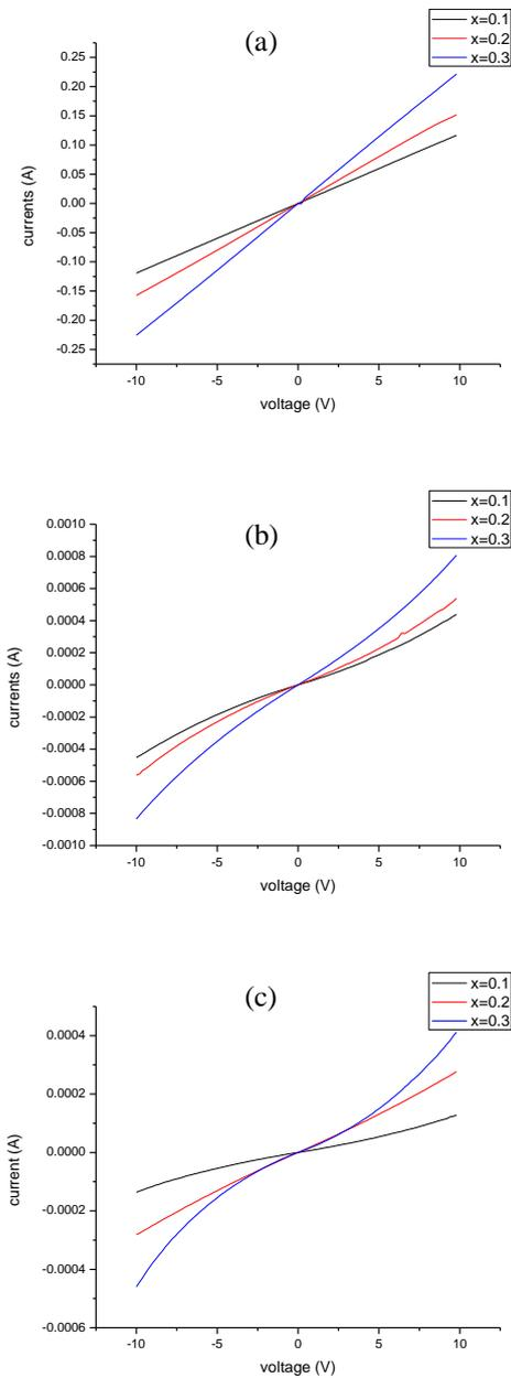
**FIGURE 5.** IV characteristics of VACNTs on MgZnO thin film with (a) aurum; (b) platinum; (c) aluminium; as a metal contact.
