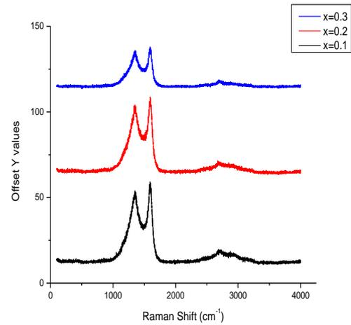
**FIGURE 4.** Raman spectroscopy showing D and G line for MWCNTs.
