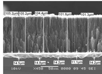
**FIGURE 2.** Vertically aligned CNTs grown on MgZnO thin film
