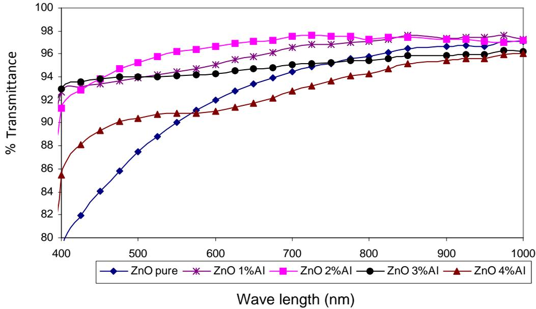
Figure 5: ZnO and ZnO:Al(1-4%) thin films transmittance spectroscopy
