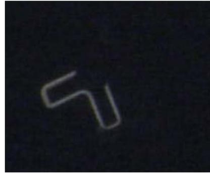
Fig. 1b. Photon emission along emitter-base junction during stress ( $V_{BE} = -8$  Volts)
