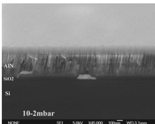
Figure 5: Cross sectional FESEM images of the AlN films synthesised under different pulverisation pressure.
