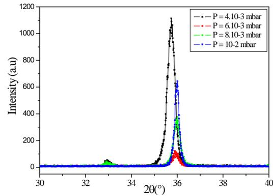
Figure 4: XRD spectra of AlN thin films deposited at different pressures
