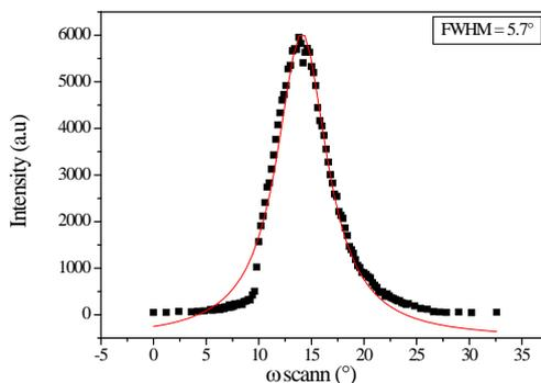
Figure 8: Rocking curve on (002) orientation of c-axis inclined AlN thin film
