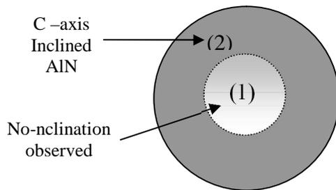
Figure 3: Schematisation of different parts of Si (100) 3" wafer
