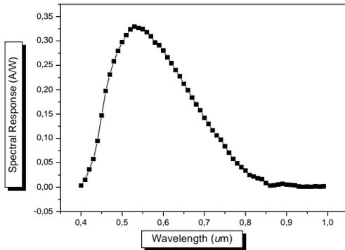
Figure 1: Spectral response of microcrystalline solar cell.
