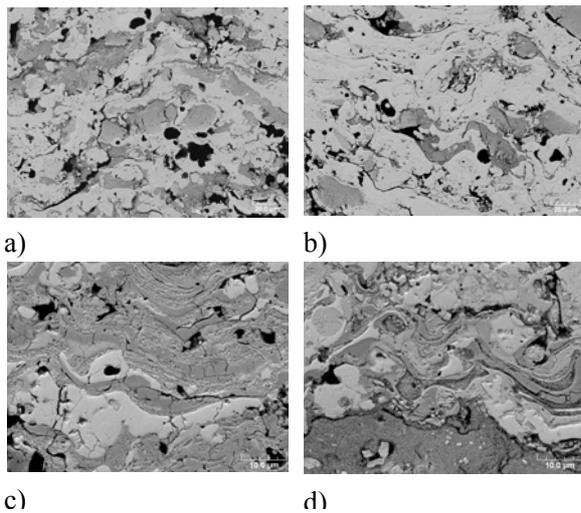
Fig. 2. SEM cross-sectional microstructure of (a) D<sub>1</sub>, (b) D<sub>2</sub>, (c) D<sub>3</sub>, (d) D<sub>30</sub> coatings.
