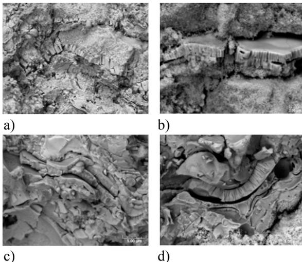
Fig. 3 fracture profile of (a) D<sub>1</sub>, (b) D<sub>2</sub>, (c) D<sub>3</sub>, (d) D<sub>30</sub> coatings.
