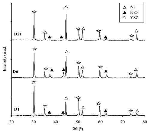
Fig. 6. X-ray diffraction of D<sub>1</sub>, D<sub>6</sub> and D<sub>21</sub> Ni-YSZ coatings.
