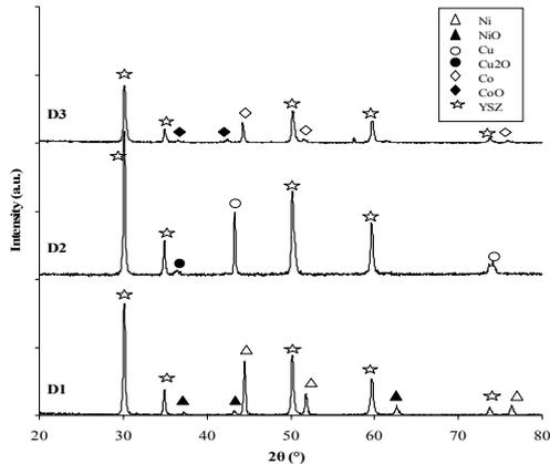
Fig. 5. X-ray diffraction of D<sub>1</sub> (Ni-YSZ), D<sub>2</sub> (Cu-YSZ) and D<sub>3</sub> (Co-YSZ) coatings.
