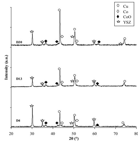
Fig. 7. X-ray diffraction of D<sub>4</sub>, D<sub>13</sub> and D<sub>30</sub> Cu-Co-YSZ coatings.
