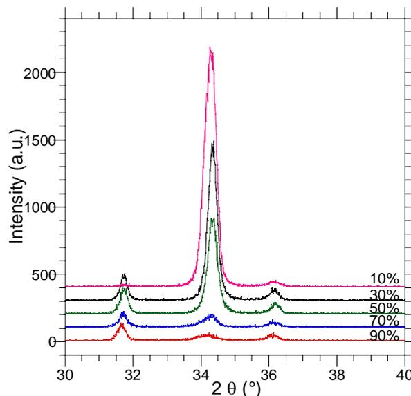
Fig.3 X-ray spectra of ZnO thin film as a function of oxygen percentage in the gas mixture
