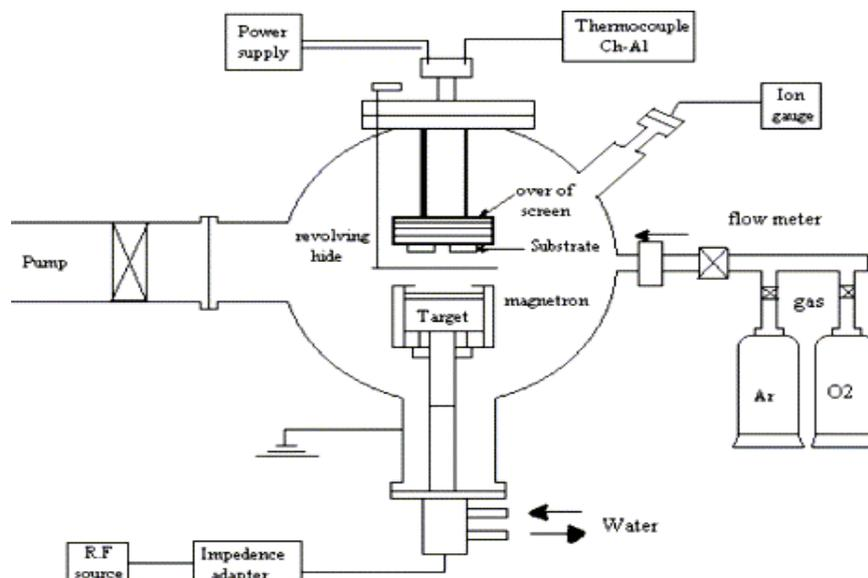
Fig.1 Radio frequency magnetron sputtering system.
