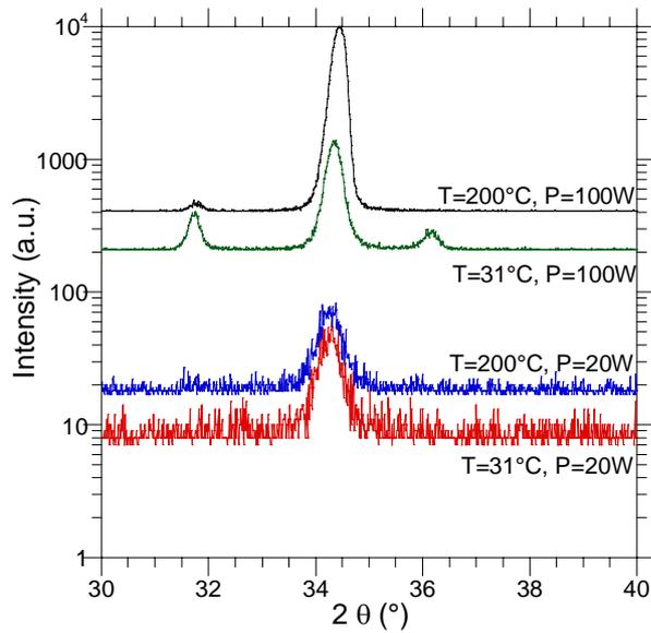
Fig.5 X-ray diffractograms of ZnO thin films as function of r.f. power, (a) at T=31°C, (b) at T=200°C.
