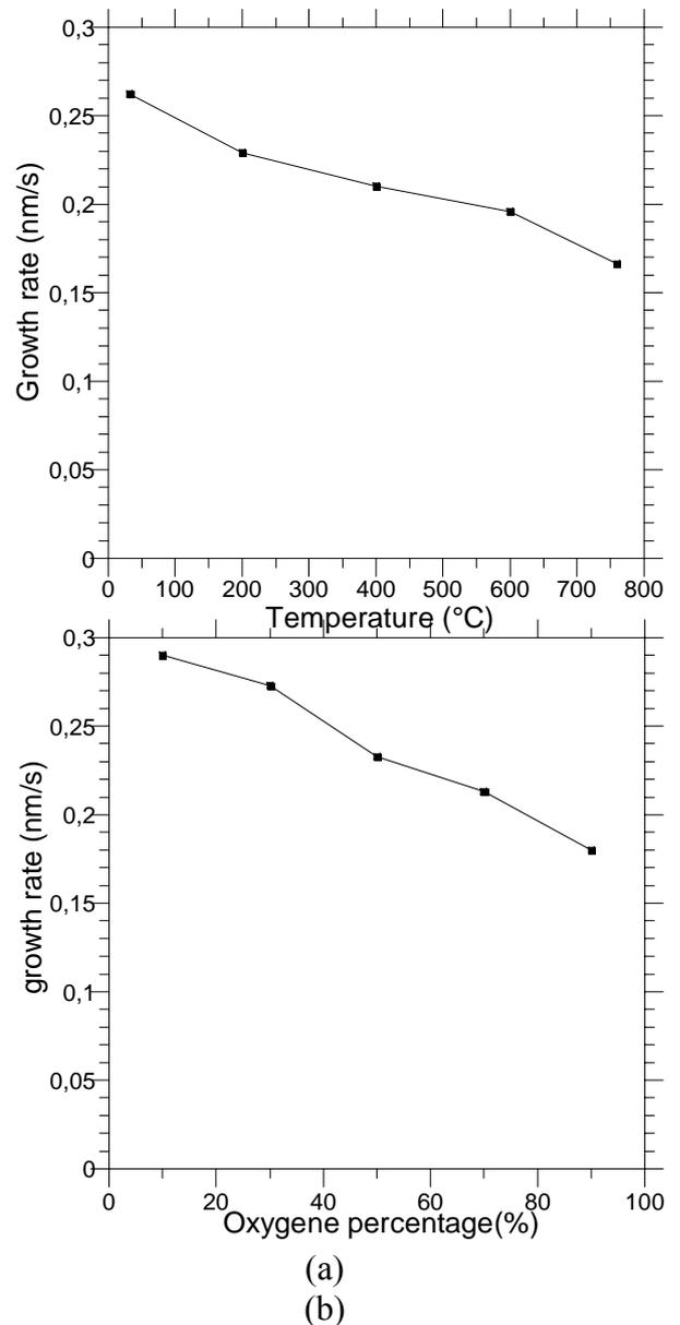
Fig.6 ZnO growth rate as function of the substrate temperature (a) and oxygen percentage in Ar/O<sub>2</sub> gas mixture (b).
