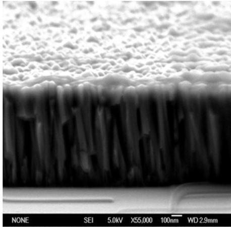
Fig.4 Cross section SEM micrograph of ZnO films at 30% of oxygen percentage in gas mixture
