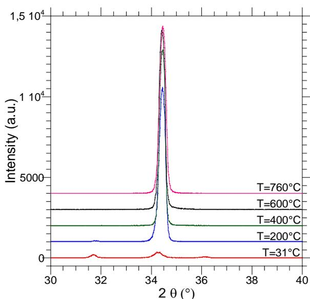
Fig.2 X-ray spectra of ZnO thin film as a function of substrate temperature.
