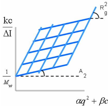
Figure 6: Zimm plot analysis of the light scattering,  $\alpha$  and  $\beta$  are adjustable parameters.
