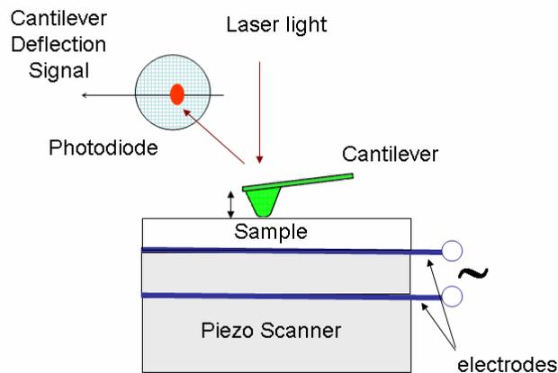
Figure 12: Principle of Atomic Force Microscopy (AFM)
