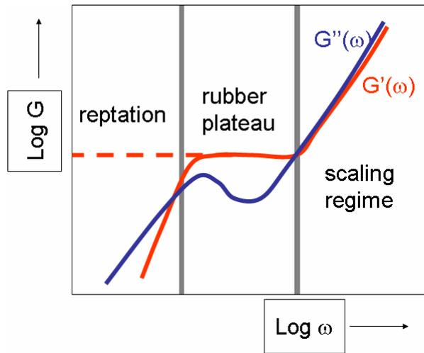
Figure 11: Viscoelastic parameter for a viscoelastic material.
