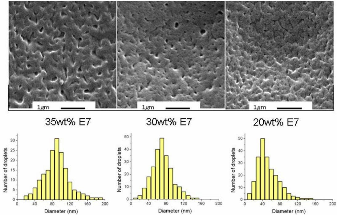
Figure 2: SEM images of PDLCs showing nanosized droplets and corresponding histograms of droplets diameter of thiol-ene / E7 at 3 concentrations of the LC.
