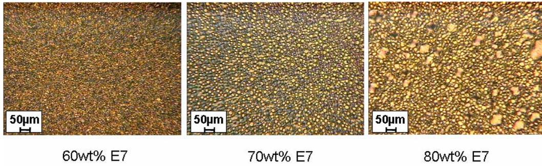
Figure 1: POM images of PDLCs showing micronsized droplets.
