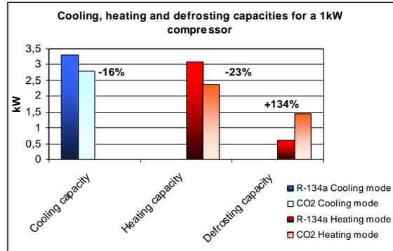
Figure 3: Performances of the HCP with R-134a or CO<sub>2</sub> as working fluid
