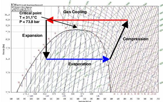
Figure 2: Transcritical cycle on the Mollier diagram
