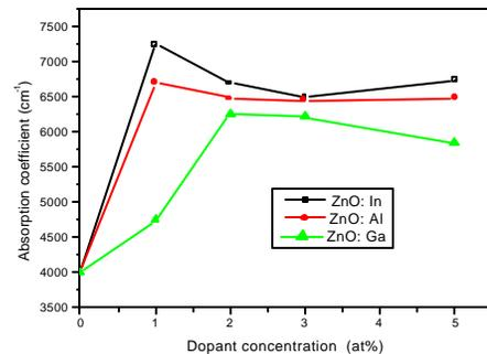
Fig n°4 : Variation of absorption coefficient with dopant concentration for the different dopants
