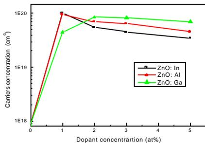
Fig n°1 : Effect of the different dopants in the carrier concentration
