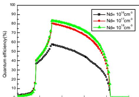
Fig. n°5 Variation of the quantum efficiency of ZnO/CdS/CIGS structure according to the doping of the ZnO layer
