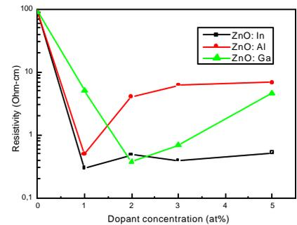
Fig n°3 : Effect of the different dopants in the resistivity
