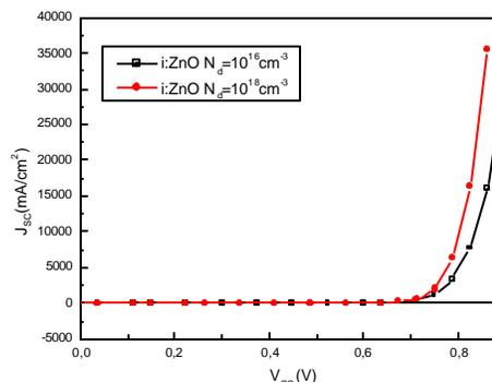
Fig.n°6: I-V characteristic of the ZnO/CdS/CIGS structure according to the doping of ZnO layer
