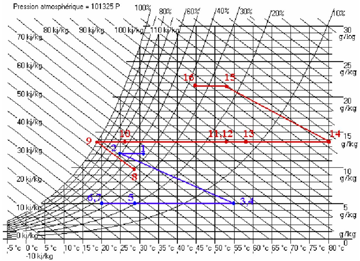
Fig. 3. Psychrometric chart – Example of the process principle
