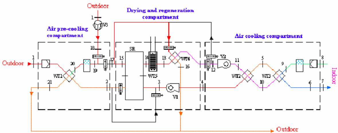
Fig. 2. Working in summer-mode with pre-cooling of air
