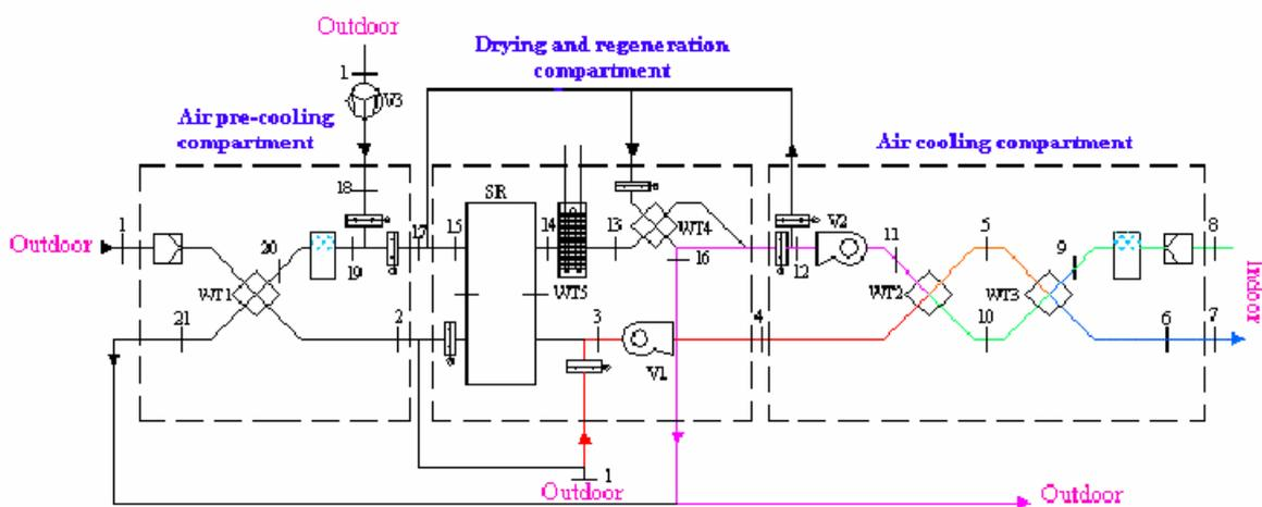
Fig. 4. Working in summer-mode without pre-cooling of air
