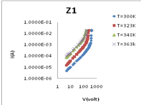
**Fig. 4:** I-V characteristics of  $Z_1$  for different temperatures
