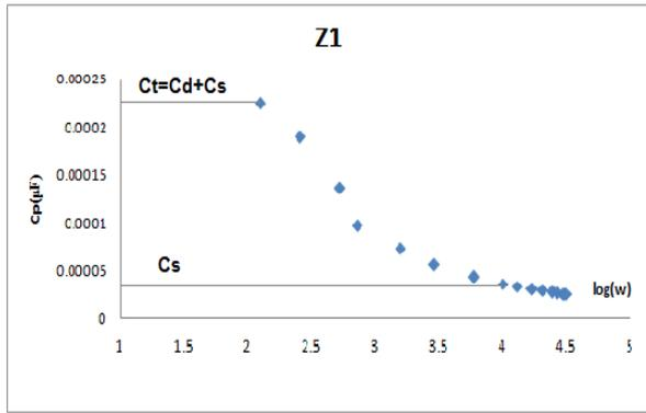
**Fig.9:** capacitance  $C_p$  as a function of  $\log(\omega)$  for  $Z_1$
