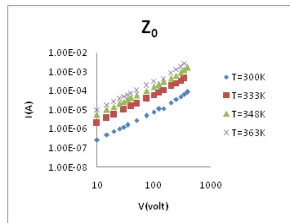
**Fig. 3:** I-V curves of  $Z_0$  with different temperatures
