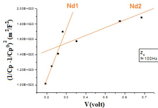
**Fig. 11:**  $(1/C - 1/C_0)^2$  vs  $V$  for sample  $Z_0$  at  $F=100\text{Hz}$ .
