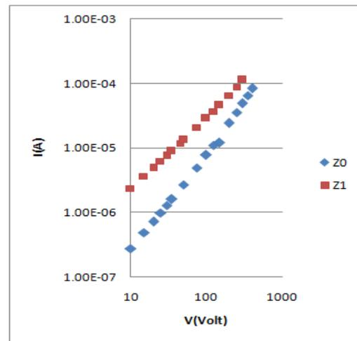
Fig. 2: I-V characteristics of samples
