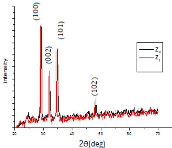
Fig. 1: XRD patterns of Z<sub>0</sub> and Z<sub>1</sub>
