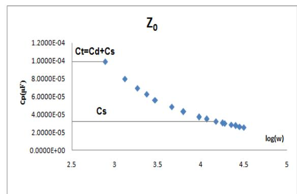
**Fig. 8:** capacitance  $C_p$  as a function of  $\log(\omega)$  for  $Z_0$
