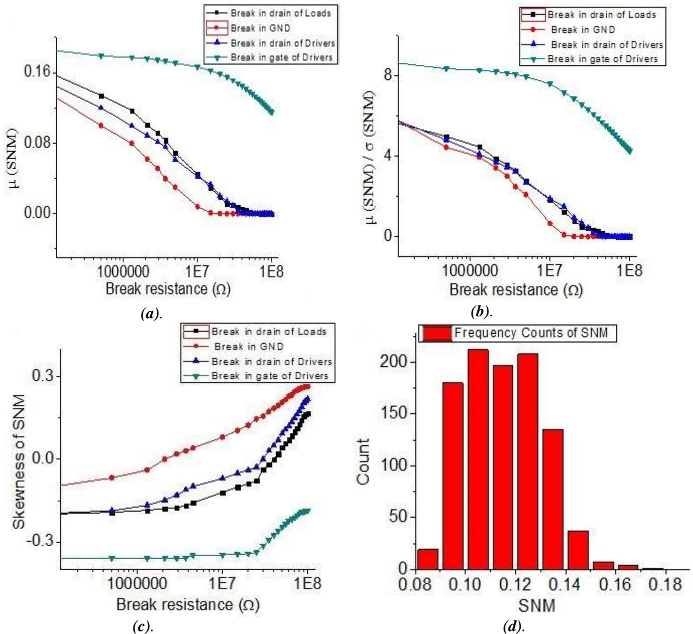
**Fig. 4** Impact of break resistance on SNM: (a):SNM mean deviation - (b):normalized standard deviation of SNM - (c):SNM skew - (d):SNM distribution.
