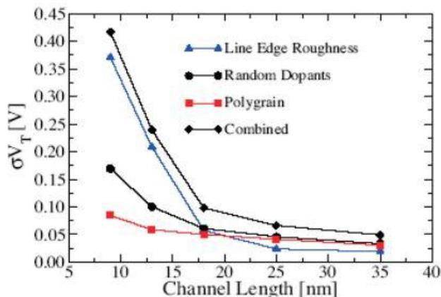
**Fig.2:** Standard deviation of threshold voltage variation vs.channel length, for square planar bulk MOSFETs. Constant gate line edge roughness (4 nm) is assumed [3].
