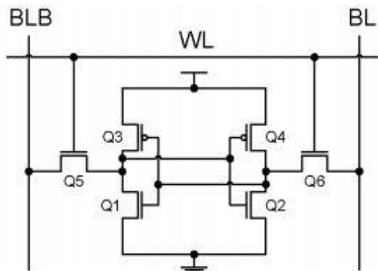
**Fig.1:** Six-transistor(6T) CMOS SRAM cell.
