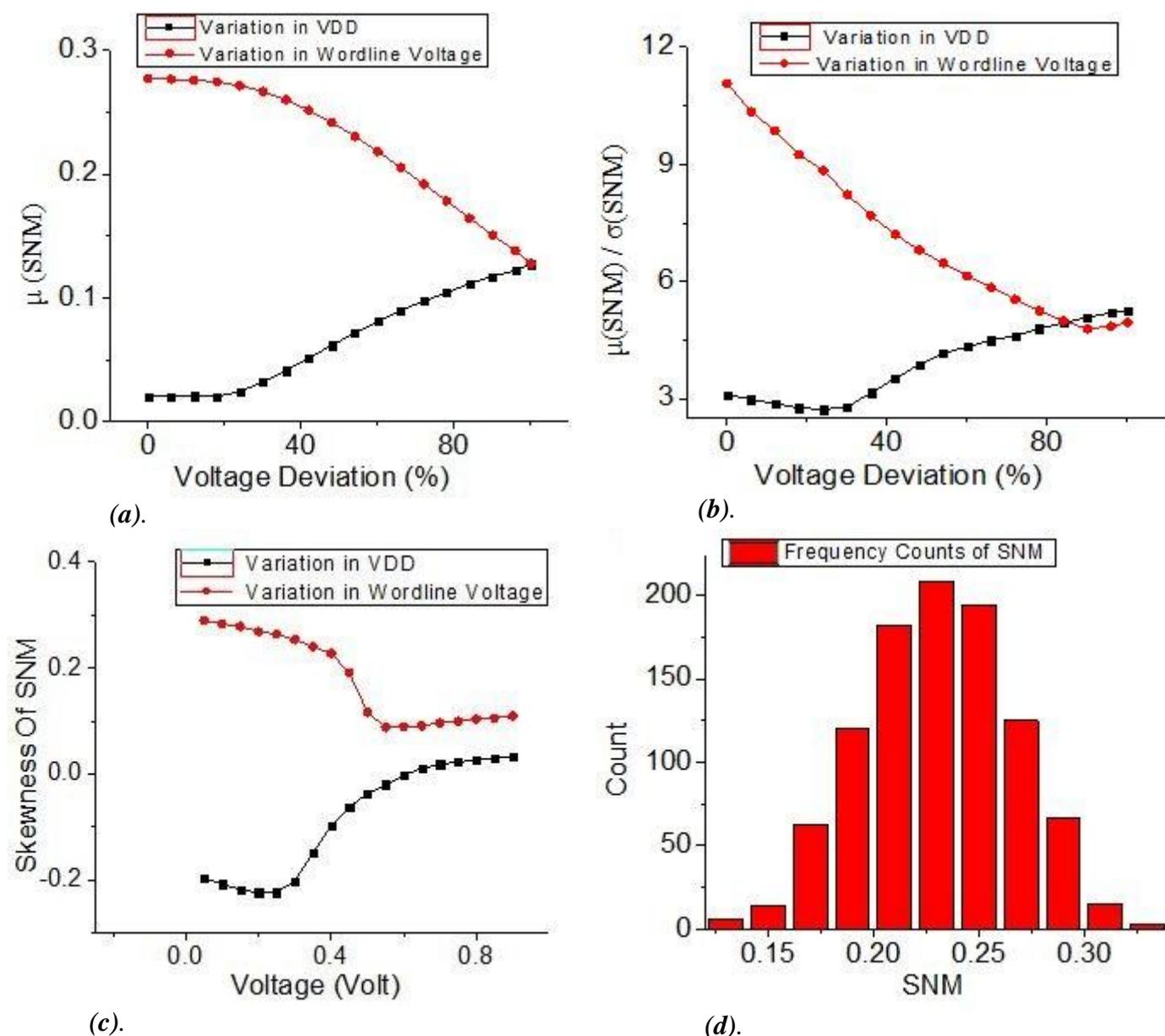
**Fig. 6:** Impact of voltage deviations on SNM: (a):SNM mean deviation - (b):normalized standard deviation of SNM - (c):SNM skew - (d):SNM distribution.
