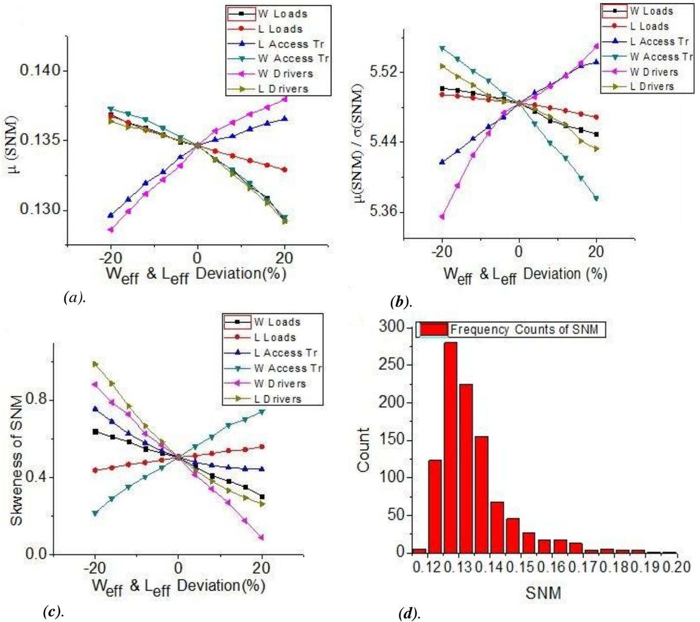
**Fig. 5:** Impact of  $W_{eff}$  and  $L_{eff}$  deviations on SNM: (a):SNM mean deviation - (b):normalized standard deviation of SNM - (c):SNM skew - (d):SNM distribution.
