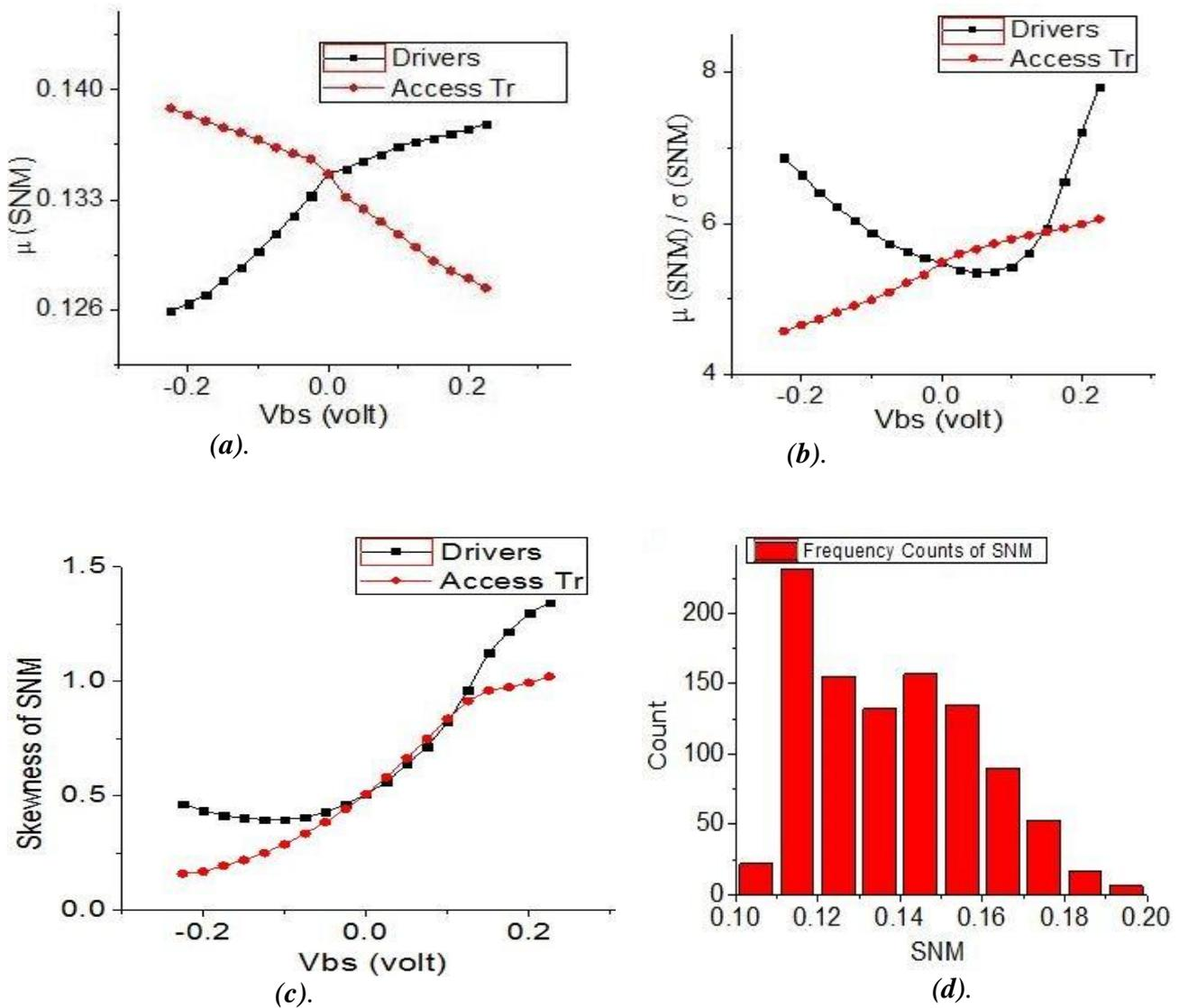
**Fig. 3:** Impact of VTH (Vbs) deviations on SNM (a):SNM mean deviation - (b):normalized standard deviation of SNM - (c):SNM skew - (d):SNM distribution.
