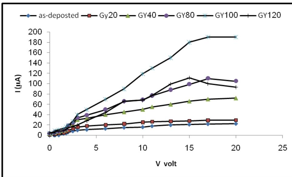
**Figure (2):** current against applied voltage for 12% Al doped CdS thin films exposed to different levels of gamma radiation doses
