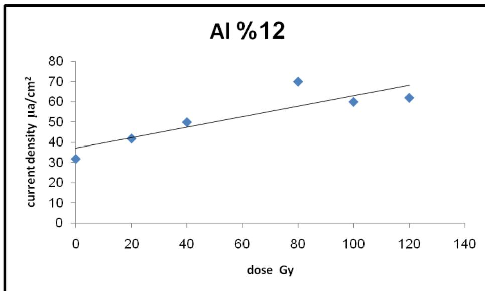
**Figure (6):** the variation of current density with the gamma doses for 12% Al rate
