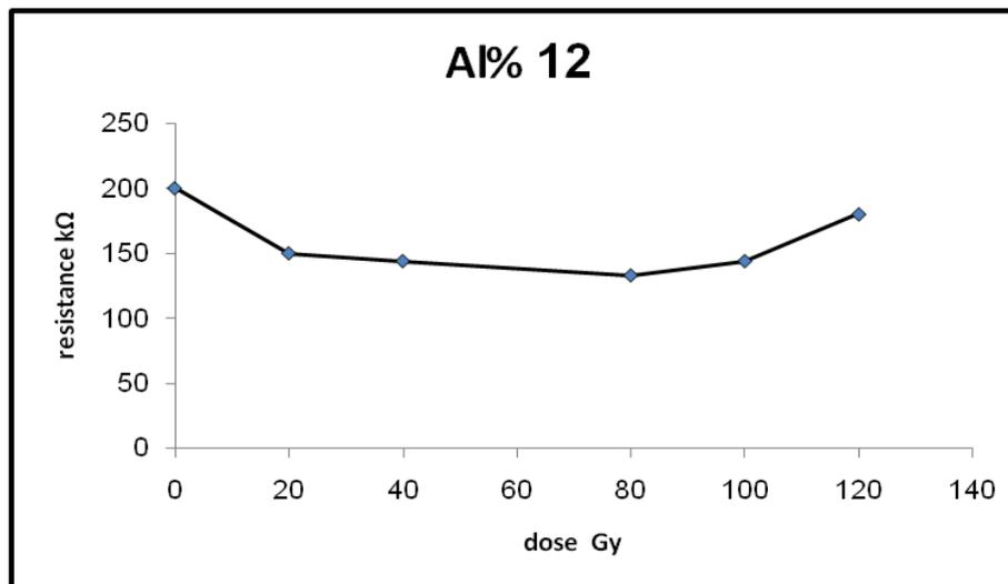
**Figure (4):** the resistance of 12% Al doped CdS films under the influence of  $\gamma$  ray irradiations
