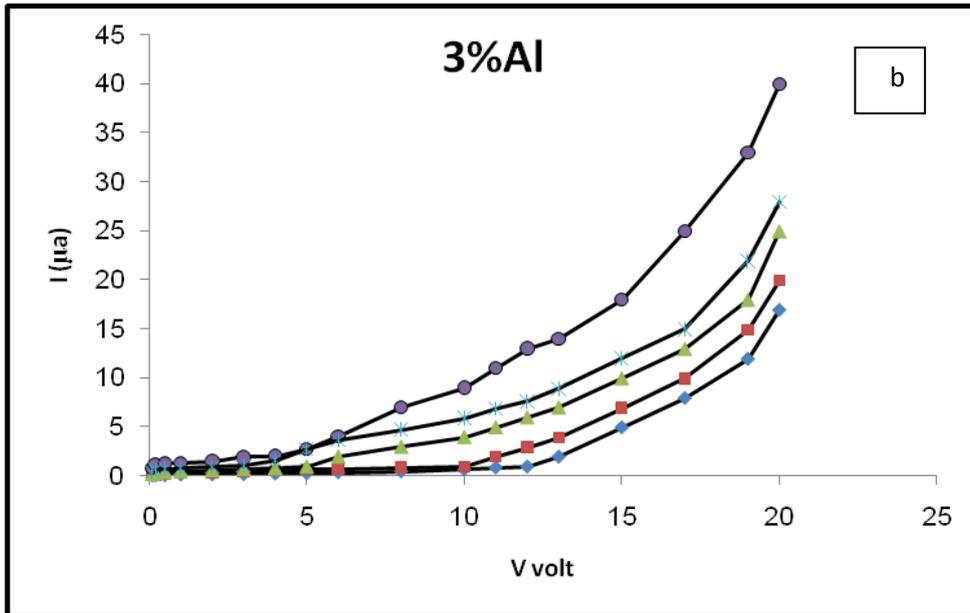
**Figure (1a,b):** current against applied voltage for the pure and 3% Al doped CdS thin films respectively exposed to different levels of gamma radiation doses
