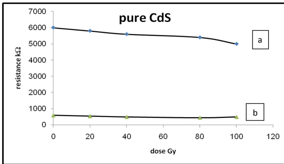
**Figure (3a,b):** resistance as function of gamma dose (a) for pure and (b) 3% Al doped CdS films
