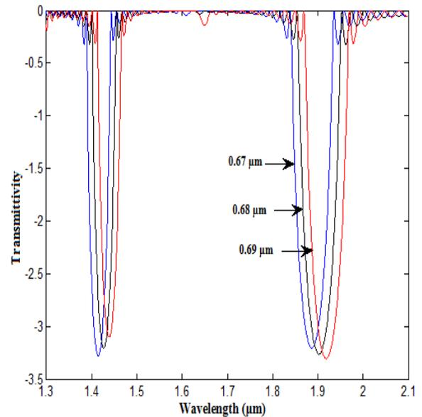
**Fig. 5.2:** Transmittivity with wavelength for oblique incidence of TE mode in presence of defect for different propagation length of second layer
