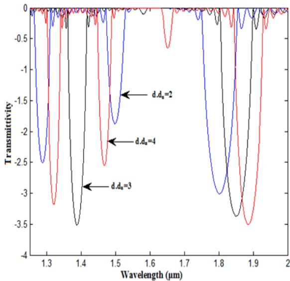
**Fig. 2:** Transmittivity with wavelength for normal incidence of TM mode in presence of defect for different defect density
