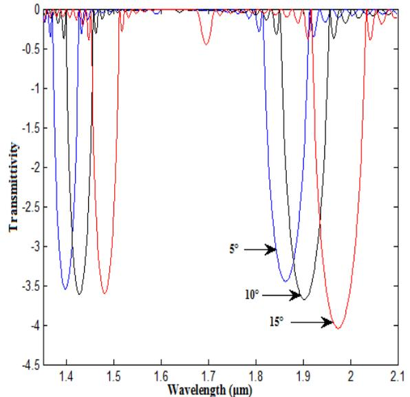
**Fig. 6.1:** Transmittivity with wavelength for oblique incidence of TM mode in presence of defect for different incident angle
