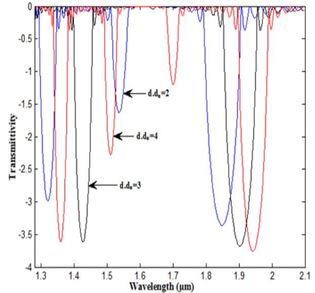
**Fig. 3.1:** Transmittivity with wavelength for oblique incidence of TM mode in presence of defect for different defect density
