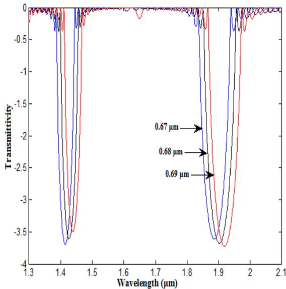
**Fig. 5.1:** Transmittivity with wavelength for oblique incidence of TM mode in presence of defect for different propagation length of well layer
