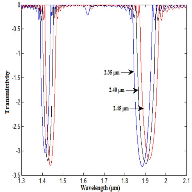
**Fig. 4.2:** Transmittivity with wavelength for oblique incidence of TE mode in presence of defect for different propagation length of barrier layer
