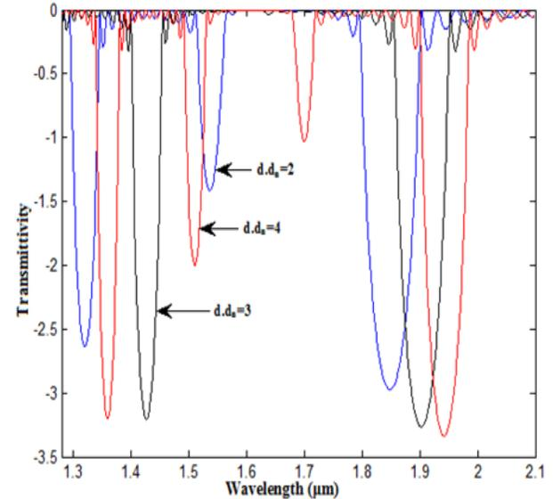
**Fig. 3.2:** Transmittivity with wavelength for oblique incidence of TE mode in presence of defect for different defect density
