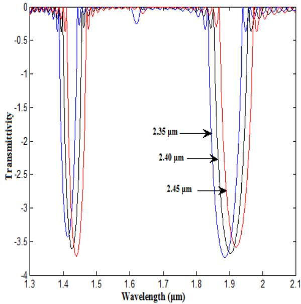
**Fig. 4.1:** Transmittivity with wavelength for oblique incidence of TM mode in presence of defect for different propagation length of barrier layer
