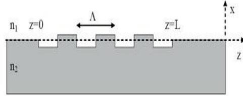
**Figure 1:** Periodic corrugation in one of the core-cladding interfaces. The grating is single mode, and we make the assumption that the only significant coupling is between counter propagating guided modes
