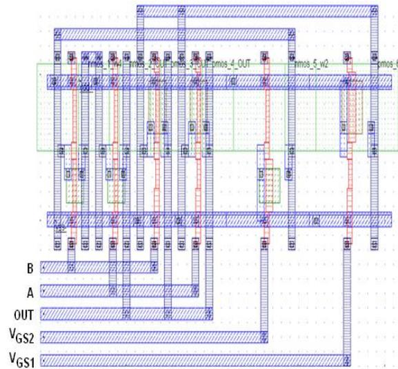
**Figure 4:** Layout of a two input NAND gate using SCCMOS technique
