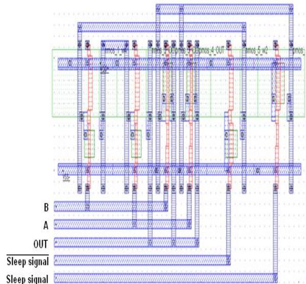
**Figure 3:** Layout of a two input NAND gate using MTCMOS technique
