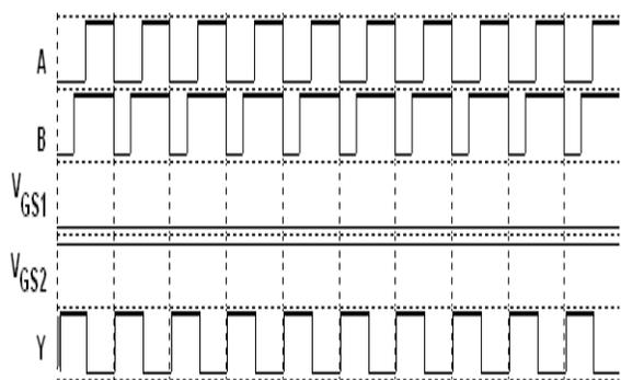
**Figure 6:** Output waveform of a two input NAND gate using SCCMOS technique
