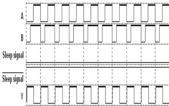
**Figure 5:** Output waveform of a two input NAND gate using MTCMOS technique
