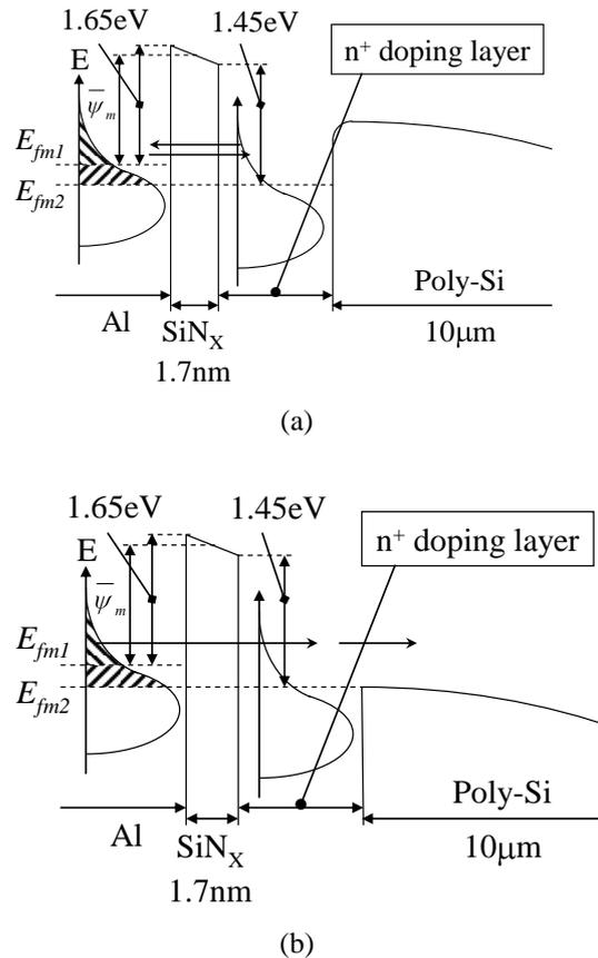
Fig. 3: Band diagram of TDTFT at a high temperature without (a) and with (b) application of bias voltage.
