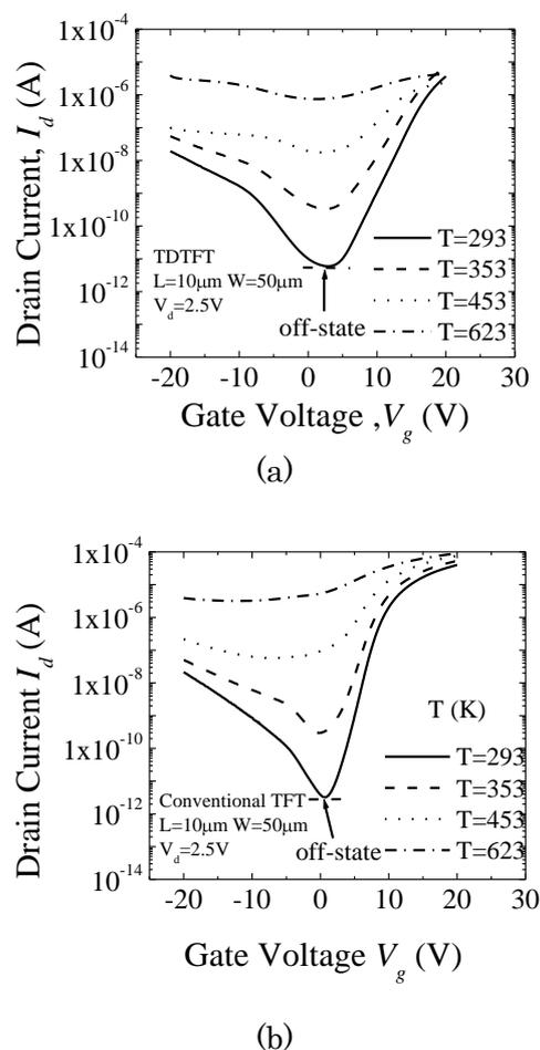
**Fig. 4:** The  $I_d$ - $V_g$  characteristics of the TDTFT (a) and conventional TFT (b).
