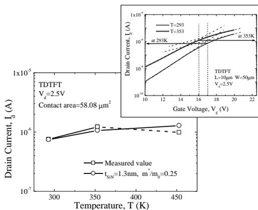
**Fig. 5:** Relationships between calculated and measured drain currents of TDTFT for conditions.
