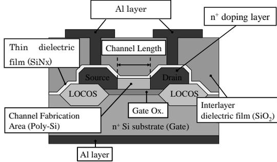
**Fig. 1:** Cross section view of bottom-gate TDTFT.
