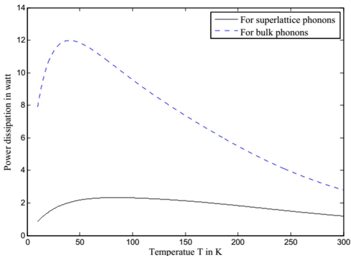
**Fig. 4:** Variation of power dissipation with temperature in MOSFET
