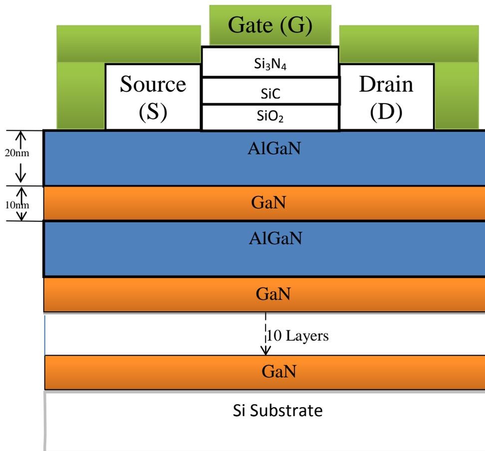
Fig. 5: Structure of superlattice MOSFET
