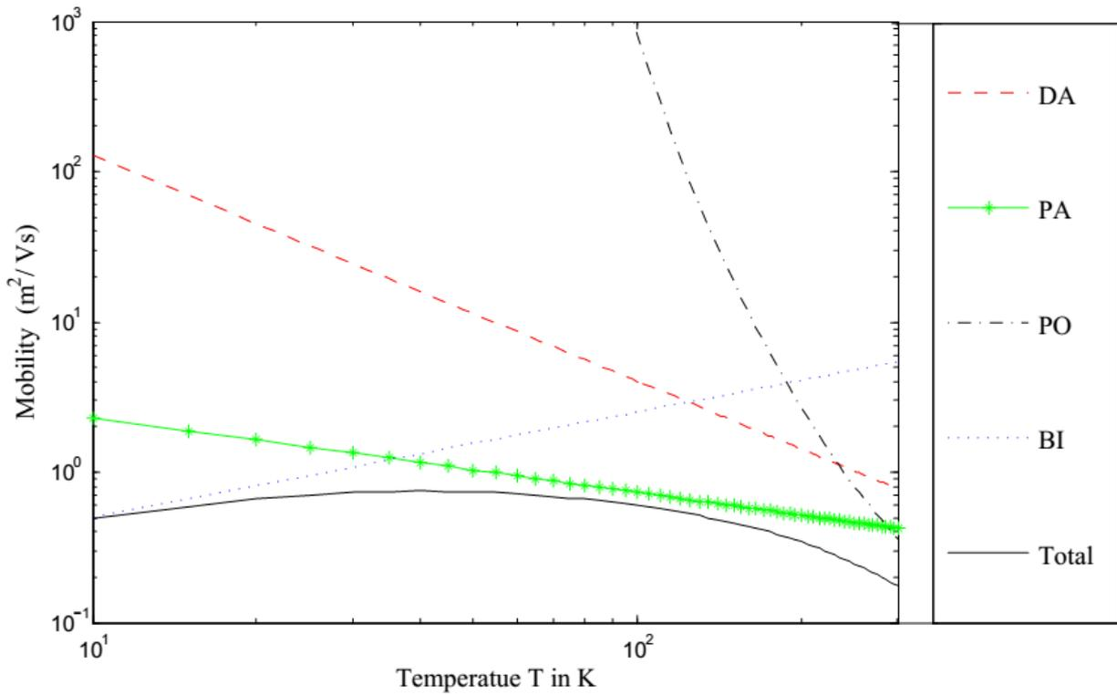
**Fig. 2:** Mobility of electron versus temperature for bulk GaN
