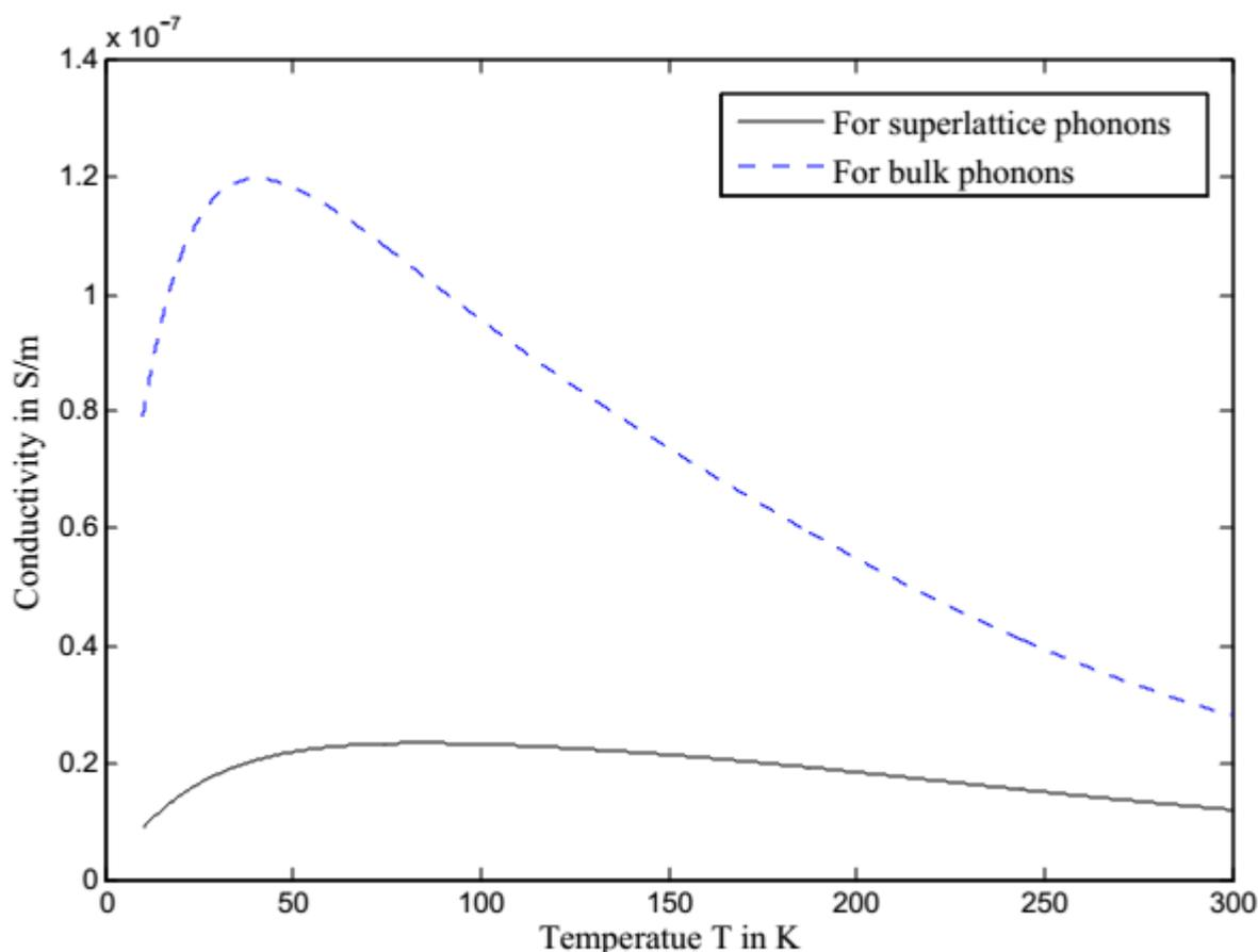
**Fig. 3:** Variation of conductivity with lattice temperature  $T$  in AlGaIn/GaN MOSFET
