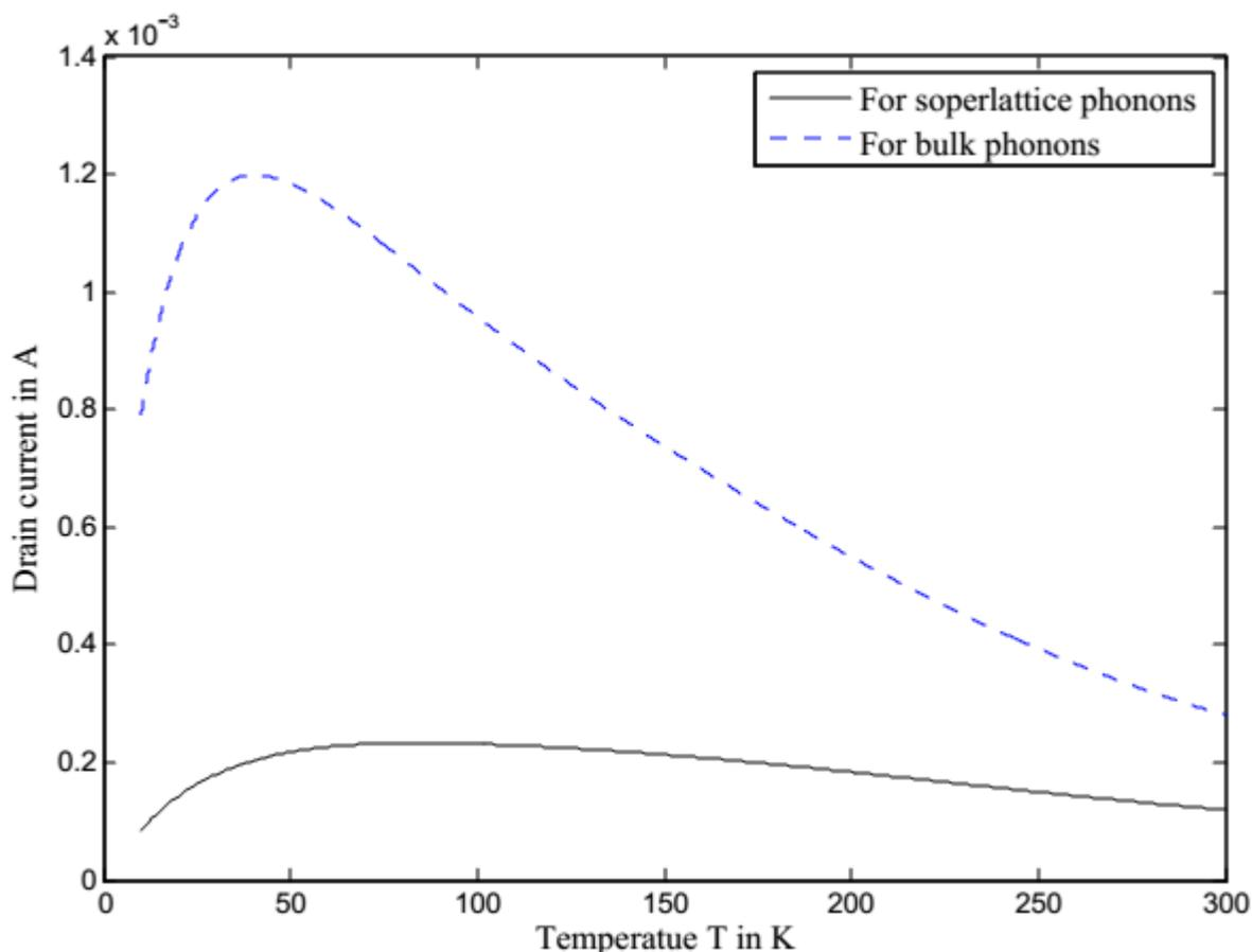
**Fig. 6:** Drain current versus lattice temperature characteristics for both superlattice and bulk phonons
