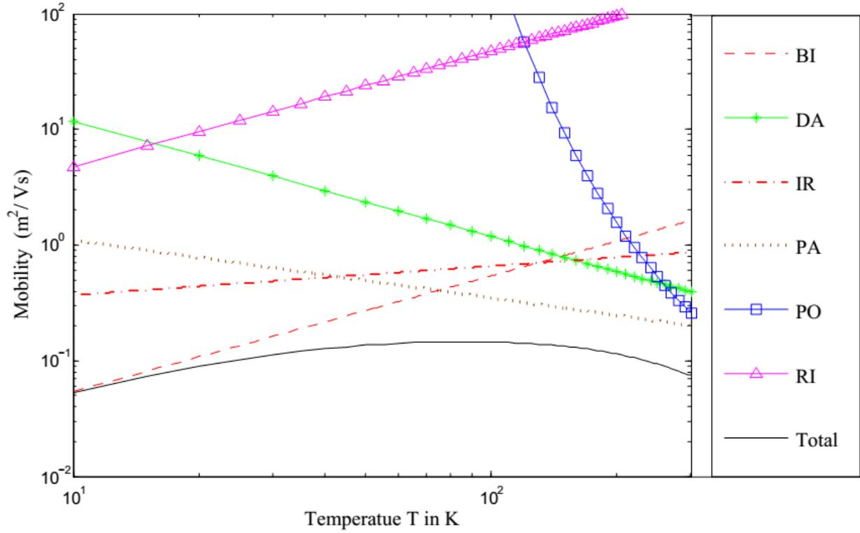
**Fig. 1** Mobility of electrons versus temperature for a GaN QW of thickness (L) 50 Å
