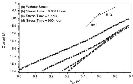
Figure 1 : Variation of the I-V characteristics for different stress times
