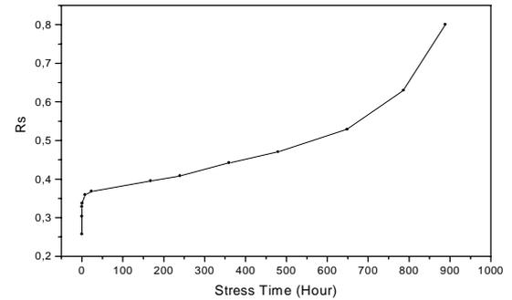
Figure 3 : Evolution of the series resistance with time during the stress time
