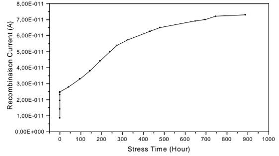
Figure 2 : Evolution of the recombination current versus the stress time
