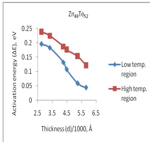
**Fig. 4:** Plot of activation energy ( $\Delta E$ ) versus thickness ( $d$ ) of Zn-Te thin films in the temperature range of 301 K to 423 K.
