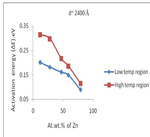
**Fig. 5:** Plot of activation energy ( $\Delta E$ ) versus at.wt.% of Zn in Zn-Te films in the temperature range of 287 K to 423 K.
