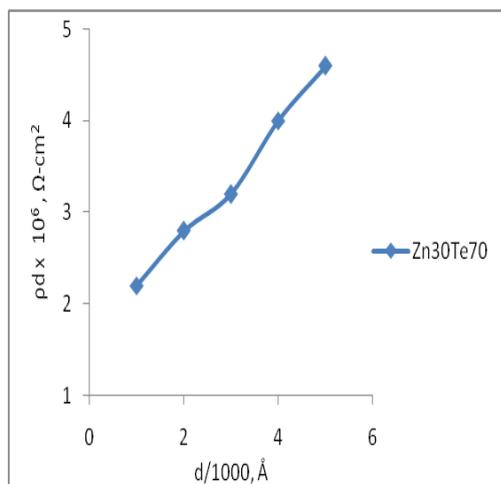
**Fig. 9:** Plot of ( $\rho d$ ) versus thickness ( $d$ ) of Zn-Te films in the temperature range of 271 K to 423 K.
