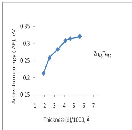
**Fig. 3:** Plot of activation energy ( $\Delta E$ ) versus thickness ( $d$ ) of Zn-Te thin films in the temperature range of 287 K to 301 K.
