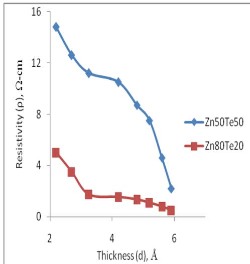
**Fig. 6:** Plot of resistivity ( $\rho$ ) versus thickness ( $d$ ) of Zn-Te films at 313 K in the temperature range of 301 K to 423 K.
