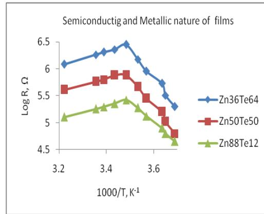
**Fig. 1:** Plot of Log(R) versus 1/T of Zn-Te thin films in the temperature range of 271 to 301 K.
