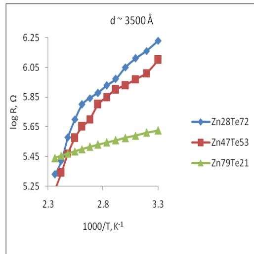
**Fig. 2:** Plot of Log(R) versus 1/T of Zn-Te thin films in the temperature range of 301 to 423 K.
