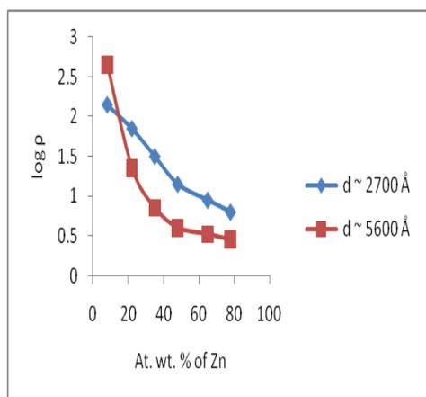
**Fig. 8:** Plot of resistivity ( $\rho$ ) versus at.wt.% of Zn in Zn-Te films at 313 K in the temperature range of 301 K to 423 K ( semiconductor region).
