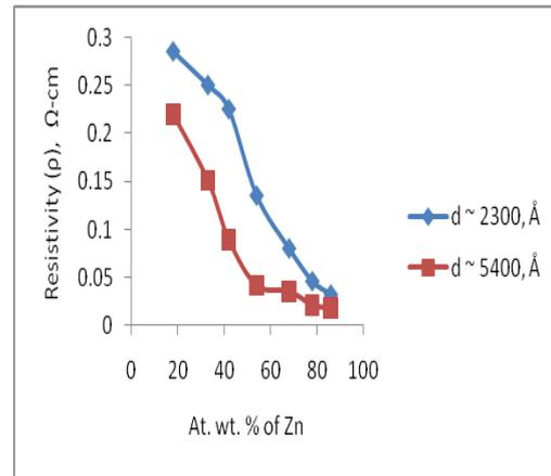
**Fig. 7:** Plot of resistivity ( $\rho$ ) versus at.wt.% of Zn in Zn-Te films at 273 K in the temperature range of 271 K to 287 K (metallic region).
