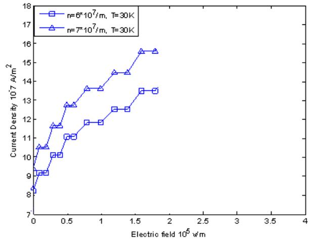
**Fig. 3:** Current Density and electric field Characteristics of 1D GaN Quantum well wire
