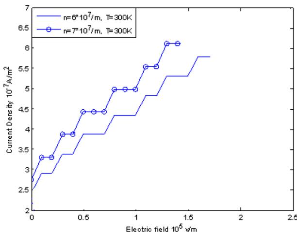
**Fig.2:** Current Density and electric field Characteristics of 1D GaN Quantum Well Wire.
