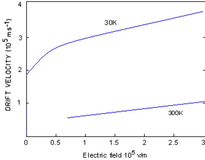
**Fig 1:** Variation of drift velocity with electric field in a quantum well wire at lattice temperature of 30K and 300K.
