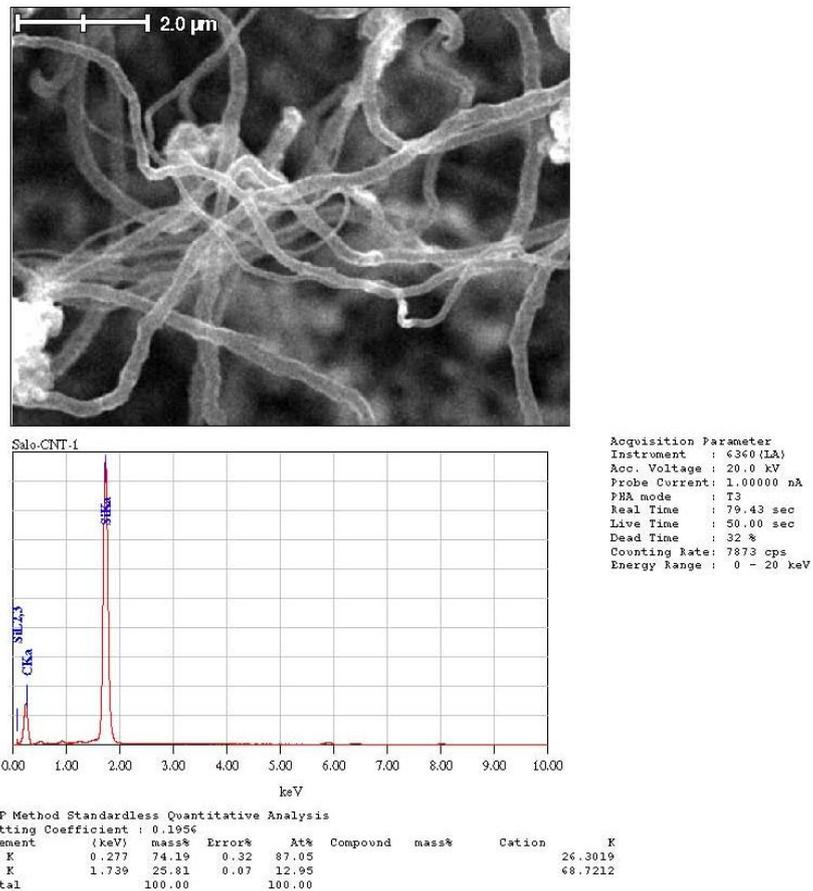
**Figure 7:** EDX spectra of CNTs grown in this study showing ~87% atomic percentage of carbon.
