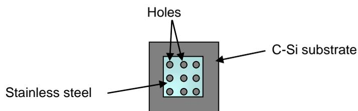
**Figure 3:** The crystal silicon substrate covered by stainless steel plate with holes
