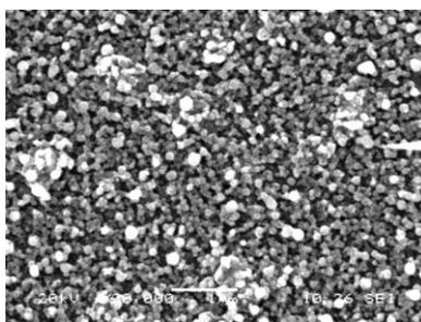
**Figure 2:** SEM micrograph showing the formation of micro-crystalline graphite having size ~ 0.1 – 0.2 micrometer.
