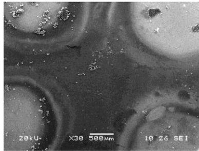
**Figure 4:** SEM micrograph showing the variation in amount of deposition with respect to the hole in the metal plate kept above the substrate
