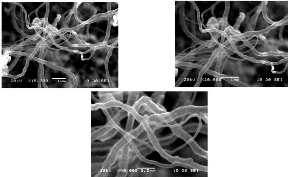
**Figure 6:** Typical CNTs deposited in this study with average diameter of ~200 nm.
