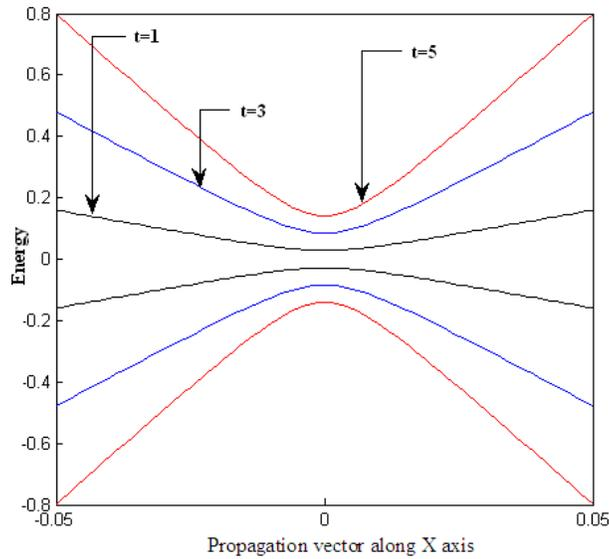
**Fig 6:** Band structure of semiconducting SWCNT with radius 0.1 nm for different values of matrix element between neighboring carbon atoms
