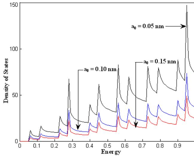
**Fig 2:** Density of states with energy for zigzag semiconducting carbon nanotube with three different radii
