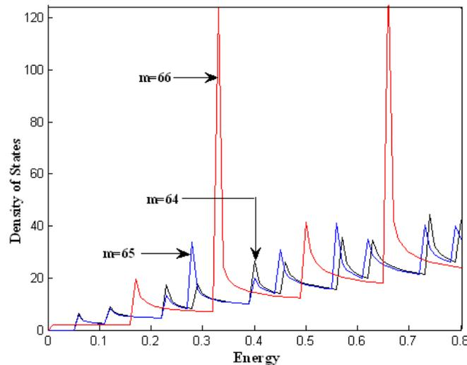
**Fig 1:** Density of states with energy for zigzag CNT with three different lattice indices having 0.1 nm radius
