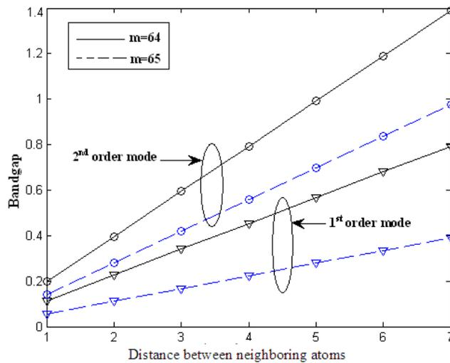
**Fig 7:** Bandgap with distance between neighboring atoms for two different semiconducting tubes for the lowest two modes
