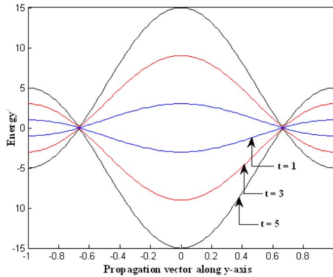
**Fig 4:** Band structure for semiconducting nanotube with radius 0.1 nm for different values of matrix elements between neighboring carbon atoms
