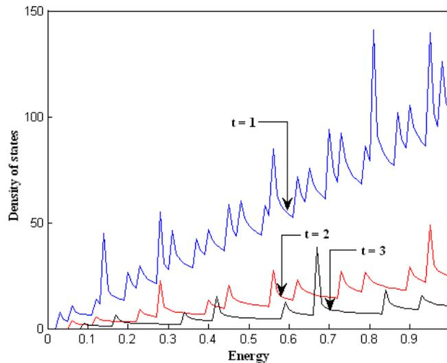
**Fig 5:** Density of states with energy for semiconducting SWCNT with radius 0.1 nm for different values of matrix element between neighboring carbon atoms
