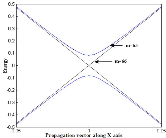
**Fig 3:** Band structure for lowest subband of metallic and semiconducting carbon nanotube
