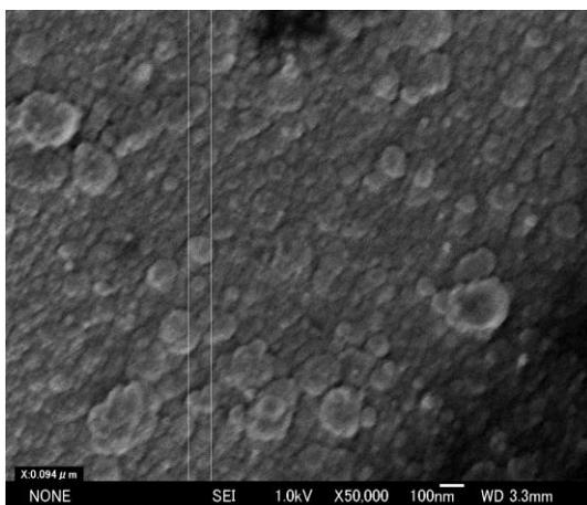
**Fig. 2:** SEM image of a clustered carbon film grown using cathodic arc process.
