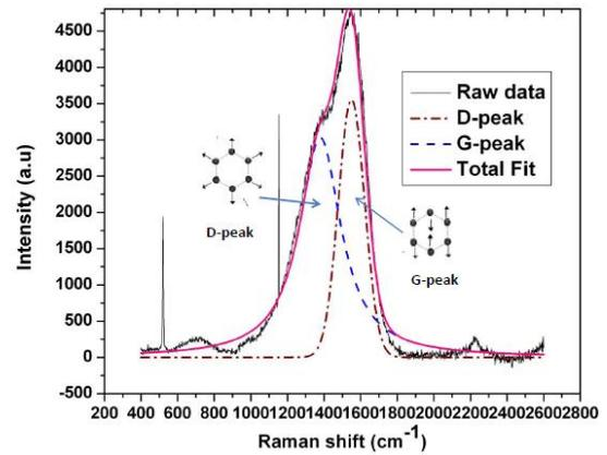
**Fig. 3:** Raman response of a clustered carbon film.
