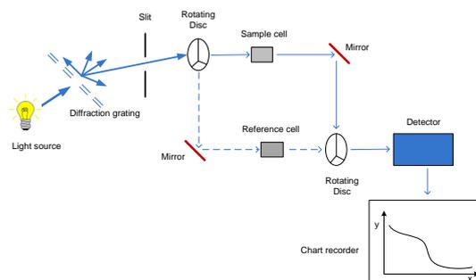
**Fig. 1:** Schematic of UV-visible spectrophotometer .
