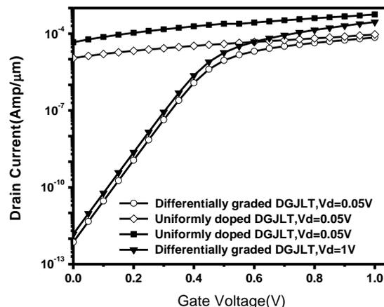
**Fig. 7:** Id-Vg plot of uniformly doped DGJLT (UD DGJLT) and differentially graded DGJLT (DG DGJLT) at different drain voltages of  $V_{DD}=0.05$  V and  $V_{DD}=1$  V,  $N_d=10^{19}$   $\text{cm}^{-3}$ ,  $L_g=60$  nm,  $T_{si}=30$  nm,  $T_{ox}=1$  nm.
