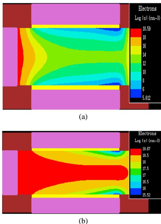
**Fig. 2:** Electron concentration in the uniformly doped DGJLT. Fig. 2(a) In off state,  $V_g=0$  V,  $V_d=1$  V; Fig. 2(b) In on state,  $V_g=1$  V and  $V_d=1$  V with  $L_g=30$  nm,  $T_{si}=12$  nm,  $N_d=10^{19}$   $\text{cm}^{-3}$ ,  $T_{ox}=1$  nm.
