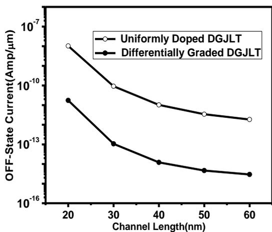
**Fig. 5:**  $I_{off}$  of uniformly doped DGJLT and differentially graded DGJLT with varying channel length with  $V_d=1$  V,  $N_d=10^{19}$   $\text{cm}^{-3}$ ,  $L_g=30$  nm,  $T_{si}=12$  nm,  $T_{ox}=1$  nm,  $T_{mid}=4$  nm,  $N_{mid}=10^{18}$   $\text{cm}^{-3}$ .
