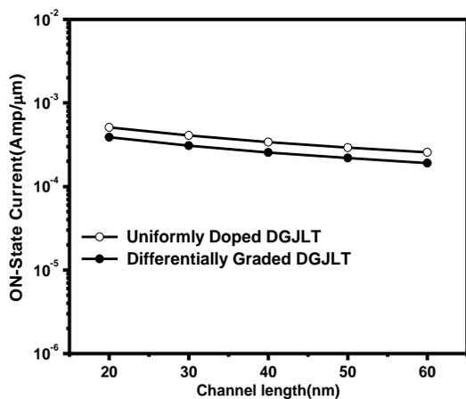
**Fig. 6:** On-state current of uniformly doped DGJLT and differentially graded DGJLT with varying channel length with  $V_d=1$  V,  $N_d=10^{19}$   $\text{cm}^{-3}$ ,  $L_g=30$  nm,  $T_{si}=12$  nm,  $T_{ox}=1$  nm,  $T_{mid}=4$  nm,  $N_{mid}=10^{18}$   $\text{cm}^{-3}$ .
