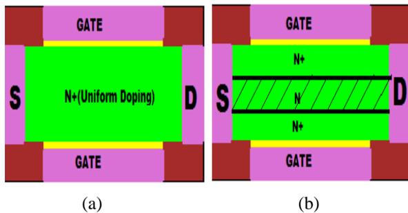
**Fig. 1:** (a) Schematic representation of the uniformly doped DGJLT and (b) schematic representation of proposed differential graded DGJLT with  $L_g = 30 \text{ nm}$ ,  $T_{si} = 10 \text{ nm}$ ,  $N_d = 10^{19} \text{ cm}^{-3}$ ,  $T_{ox} = 1 \text{ nm}$  and  $\Phi_g = 5.3 \text{ eV}$ .
