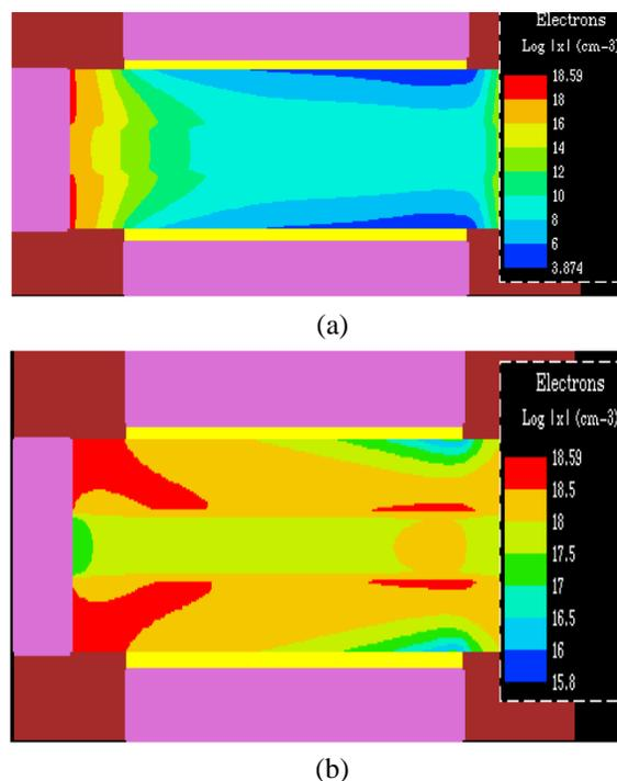
**Fig. 3:** Electron concentration of the differential graded DGJLT. Fig. 3(a) In off-state,  $V_g=0$  V,  $V_d=1$  V and Fig. 3(b) In on state,  $V_g=1$  V,  $V_d=1$  V with  $L_g=30$  nm,  $T_{si}=12$  nm,  $T_{ox}=1$  nm.
