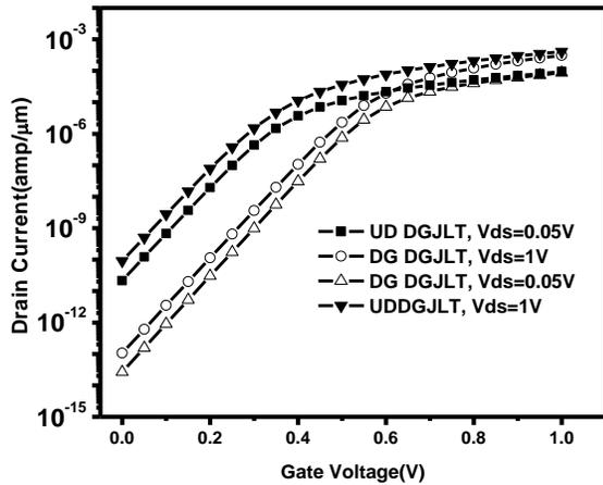
**Fig. 4:** Id-Vg plot of uniformly doped DGJLT (UD DGJLT) and differentially graded DGJLT (DG DGJLT) at different drain voltages of  $V_d=0.05V$  and  $V_d=1V$ ,  $N_d=10^{19} cm^{-3}$ ,  $L_g=30 nm$ ,  $T_{si}=12 nm$ ,  $T_{ox}=1 nm$ ,  $T_{mid}=4 nm$ ,  $N_{mid}=10^{18} cm^{-3}$ .
