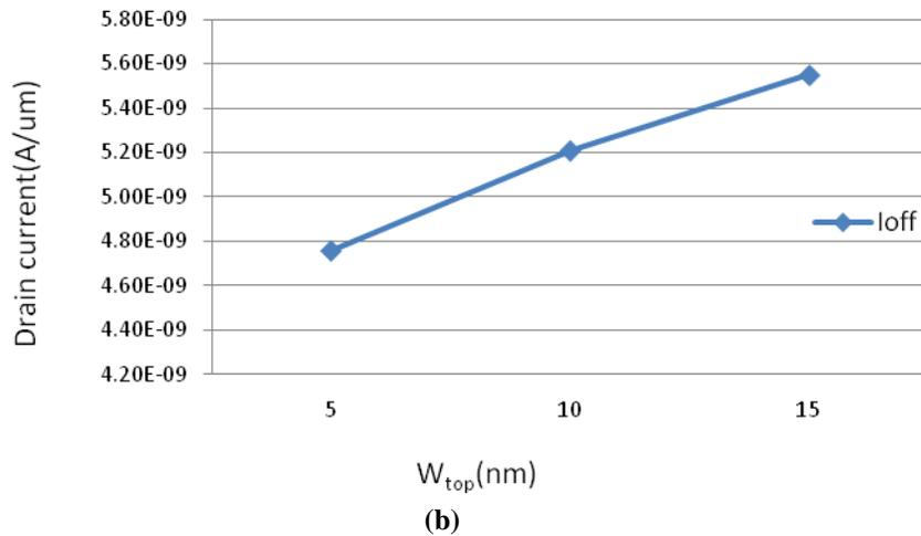
**Fig. 6:** Side-surface slope impacts I–V performance of PFinFET (a)  $I_{lin}/I_{sat}$  (b)  $I_{off}$  for different  $W_{top}$
