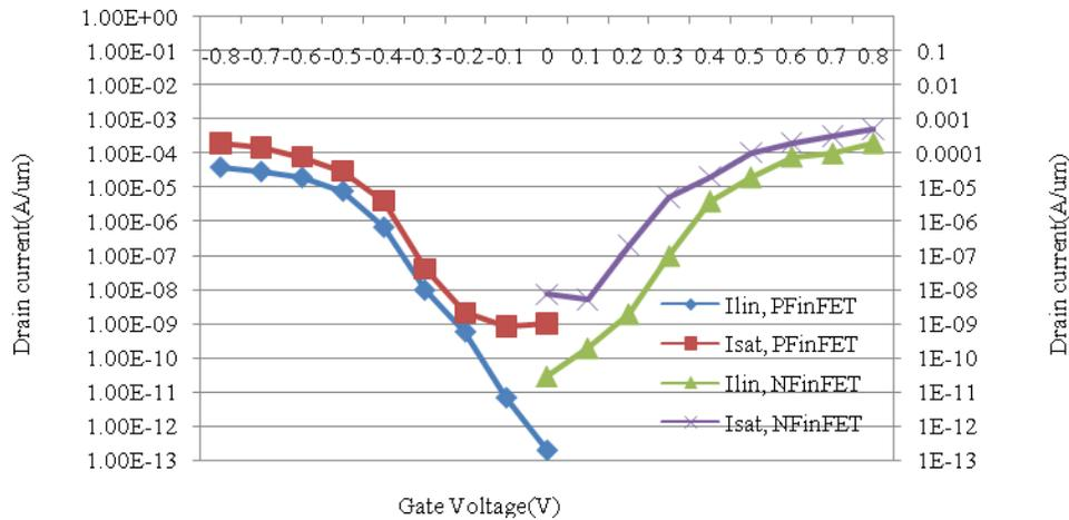
**Fig.3:** Id–Vg characteristics for NFinFET and PFinFET (Top Fin Width = 5nm)
