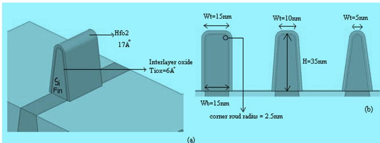
**Fig.2:** (a) Cross-sectional view of rounded corner FinFET structure for 3-D device simulation (b) Fin structure showing the variation in top fin width ( $W_{top}$ )
