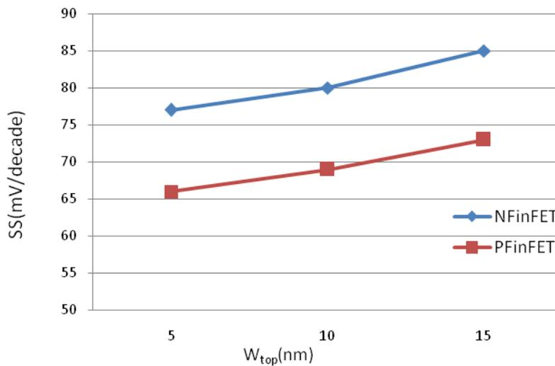
**Fig.4:** Side-surface slope impacts subthreshold slope
