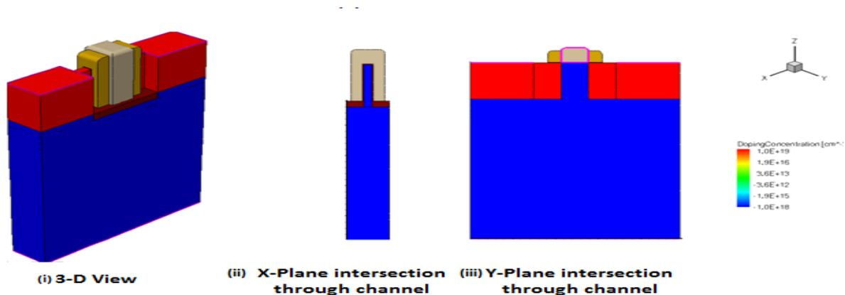
**Fig.1:** 3-D Conventional bulk FinFET Structure (without corner rounding)
