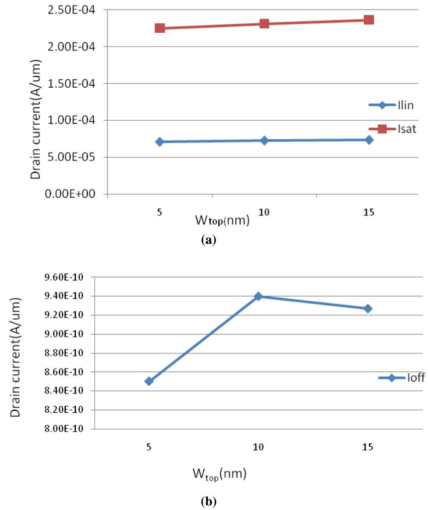
**Fig. 5** Side-surface slope impacts I-V performance of NFinFET (a)  $I_{lin}/I_{sat}$ , (b)  $I_{off}$  for different  $W_{top}$
