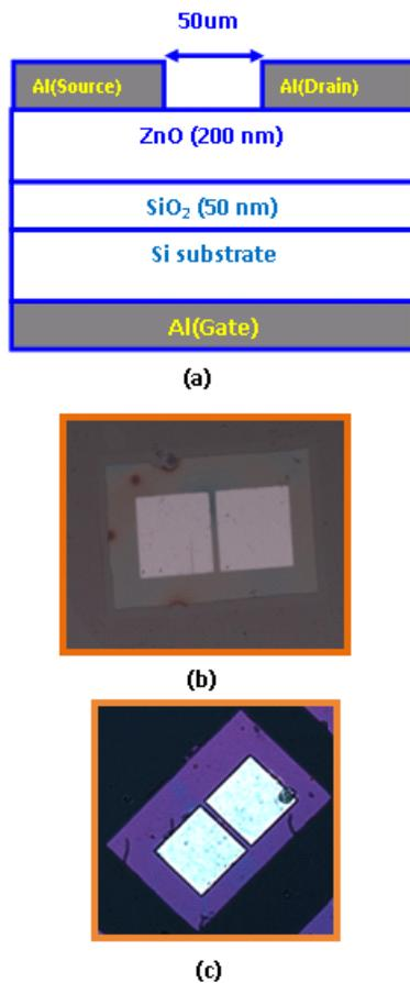
**Figure 1:** (a) The schematic structure and (b) & (c) Images of sol-gel and RF sputtered ZnO TFTs
