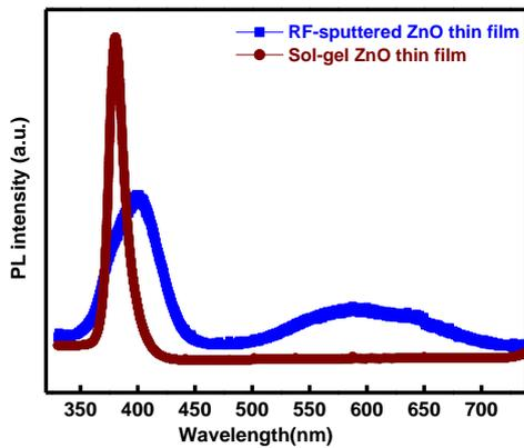
**Figure 3:** PL spectra of sol-gel and RF sputtered ZnO thin films.
