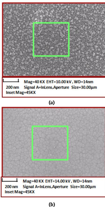
**Figure 2:** SEM images of sol-gel and RF sputtered ZnO thin films
