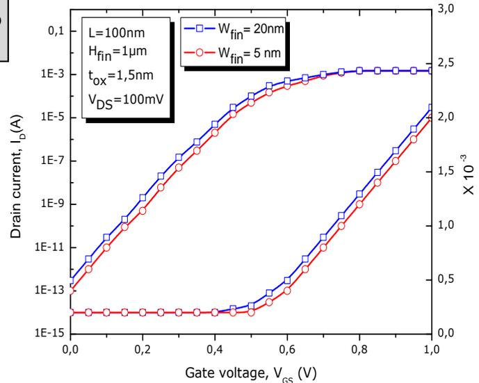
**Fig. 2:** Influence of the  $W_{fin}$  parameter in 3D simulations
