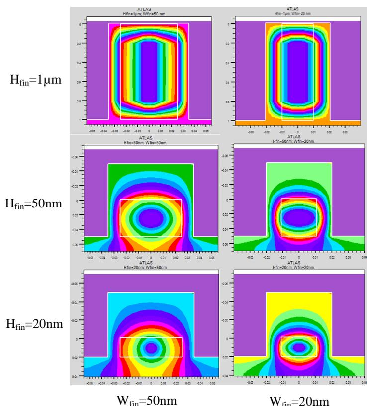
**Fig. 4:** Potential in the oxide and the silicon in the section  $y$ - $z$  for a channel length of  $1\mu\text{m}$  and a  $V_{\text{gs}} = 0.3\text{V}$
