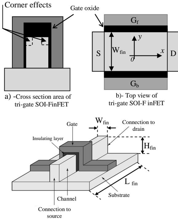
**Fig. 1:** Dimensional schematic view of tri-gate FinFET.
