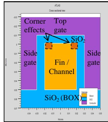
**Fig. 3-b:** Cross sectional view of tri-gate SOI-FinFET.
