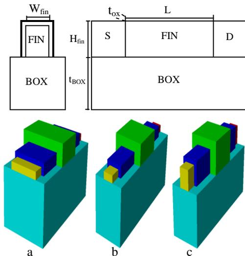
**Fig. 3-a:** The 3-D device structure generated from DevEdit3D and TonyPlot3D: a)  $H_{fin}=50nm, W_{fin}=150nm$ . b)  $H_{fin}=50nm, W_{fin}=50nm$ . c)  $H_{fin}=150, W_{fin}=50nm$
