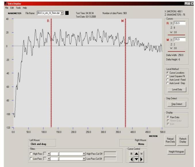
**Figure 1:** Surface Profile of the Si wafer after cleaning. desired area on wafer surface and proved its
