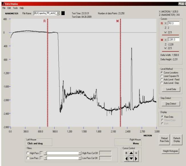
**Figure 2:** Etching Profile of Si wafer when solution concentration was 40% and exposure time was 15min.
