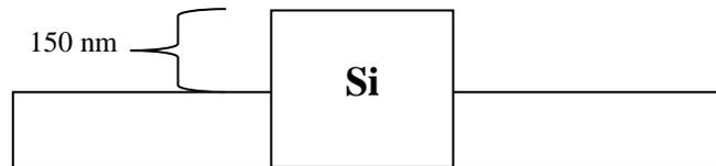
**Figure 4:** Schematic diagram of the Silicon wafer after the wet chemical etching.
