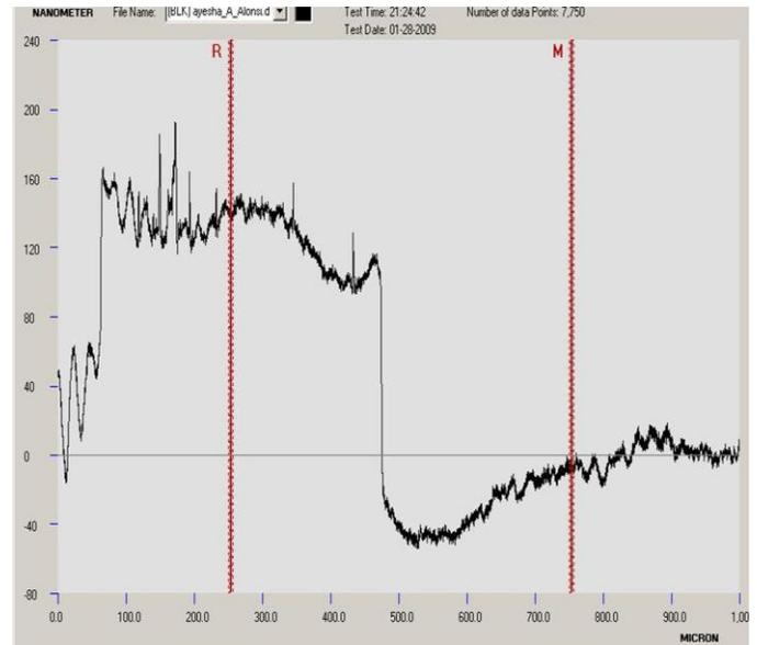
**Figure 3:** Etching profile of the Si wafer at 40% concentration of solution and exposure time was 1 min.
