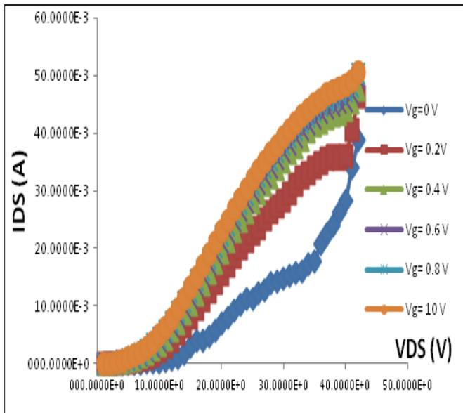
Figure 8: I-V characteristics of the Schottky Fet with positive gate voltage.
