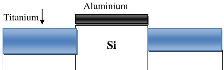
**Figure 5:** Schematic diagram of device with evaporated Titanium in the pits to form Schottky contacts.
