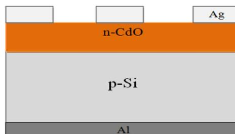
**Figure 1:** Schematic illustration of the (n-CdO/p-Si) solar cell thin film
