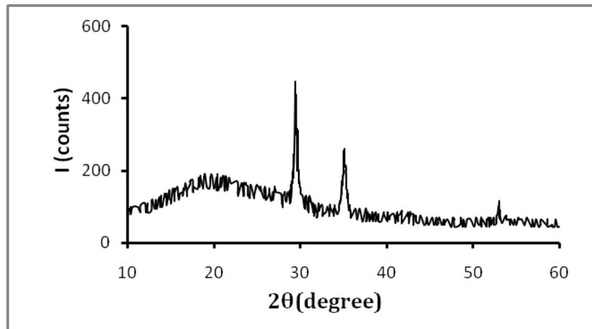
**Figure 2:** (XRD) patterns of the prepared undoped CdO
