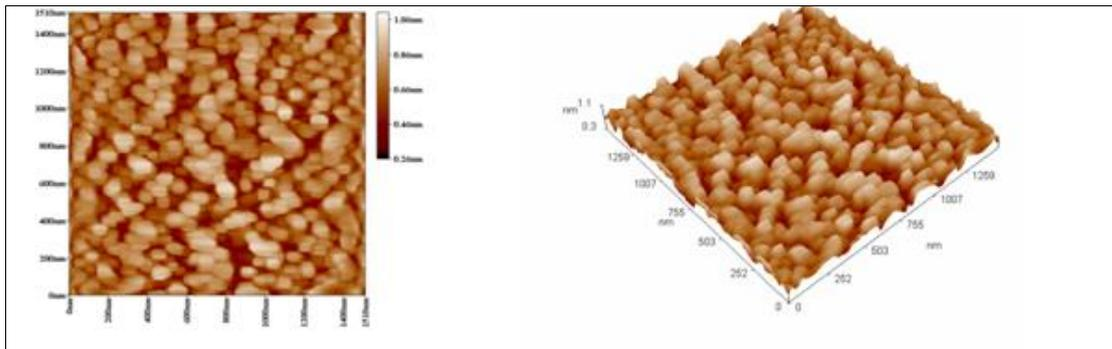
**Figure 4:** AFM image of CdO:In / Si heterojunction
