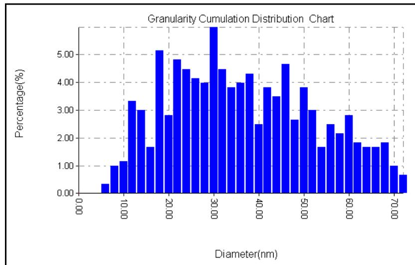
**Figure 5:** Granularity accumulation distribution of n-CdO/p-Si film
