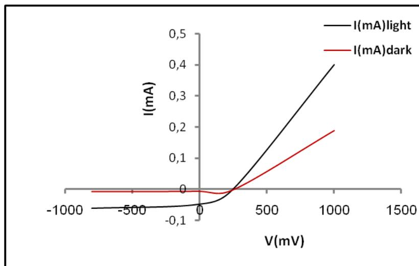
**Figure 6:** Current–Voltage characteristics of the CdO:In film under dark and illumination conditions
