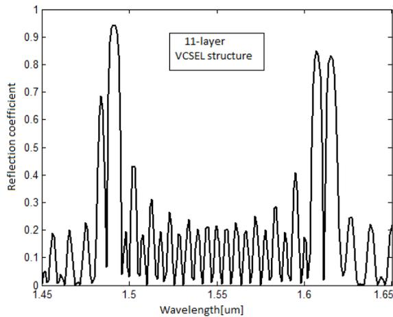
**Fig 2(a):** Reflection coefficient with wavelength for 11-layer VCSEL with  $Al_{0.4}Ga_{0.6}N/GaN$  composition
