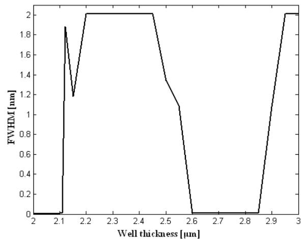
**Fig 4c:** FWHM with well thickness of MQW structure for 11-layer structure
