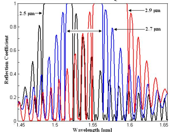
**Fig 3(b):** Reflection coefficient with wavelength for different well thickness of MQW structure
