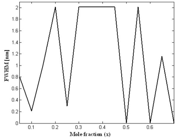
**Fig 4a:** FWHM with Al mole fraction ( $x$ ) for 11-layer structure
