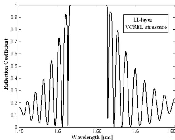
**Fig 2(b):** Reflection coefficient with wavelength for 11-layer VCSEL with  $Al_{0.6}Ga_{0.4}N/GaN$  composition
