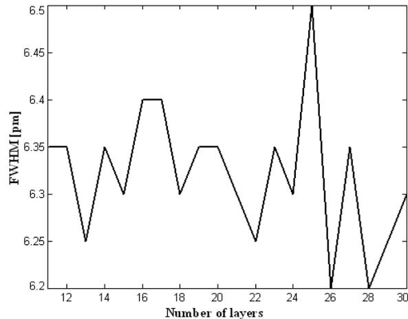
**Fig 5:** FWHM with no. of layers of MQW structure
