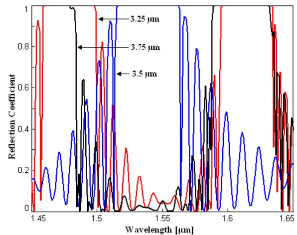
**Fig 3(a):** Reflection coefficient with wavelength for different barrier thickness of MQW structure
