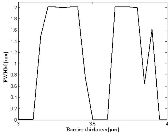
**Fig 4b:** FWHM with barrier layer width of MQW structure for 11-layer structure
