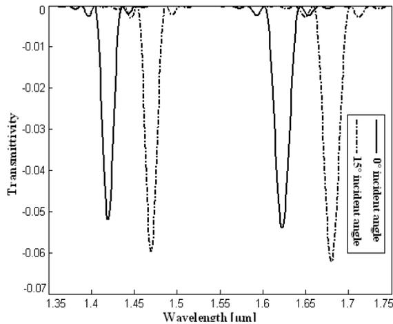
**Fig 4a:** Comparative study of transmittivity vs. wavelength of em wave for normal and oblique incidence with constant barrier and well widths and  $\text{Al}_{0.2}\text{Ga}_{0.8}\text{N}/\text{GaN}$  composition
