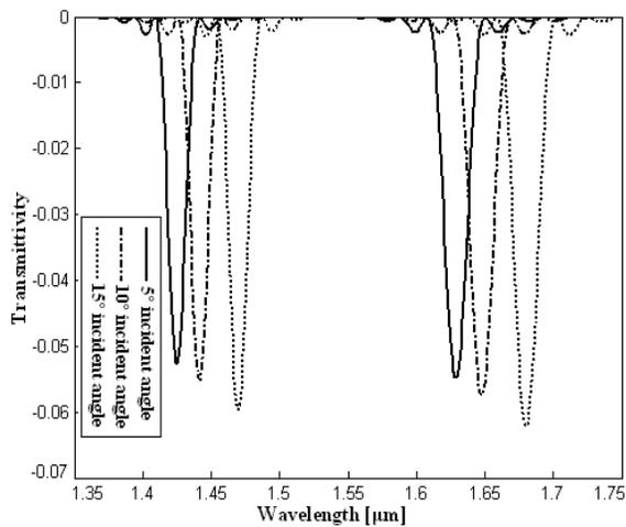
**Fig 4b:** Transmittivity vs. wavelength of em wave for different oblique incidence angle with constant barrier and well widths and  $\text{Al}_{0.2}\text{Ga}_{0.8}\text{N}/\text{GaN}$  composition
