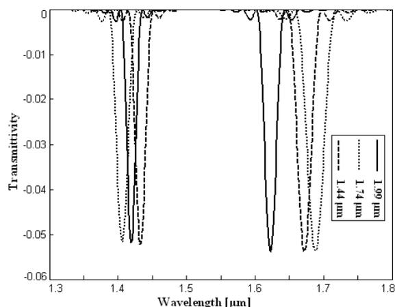
**Fig 3a:** Transmittivity vs wavelength of em wave for normal incidence for  $\text{Al}_{0.2}\text{Ga}_{0.8}\text{N}/\text{GaN}$  composition and constant well width but different barrier width
