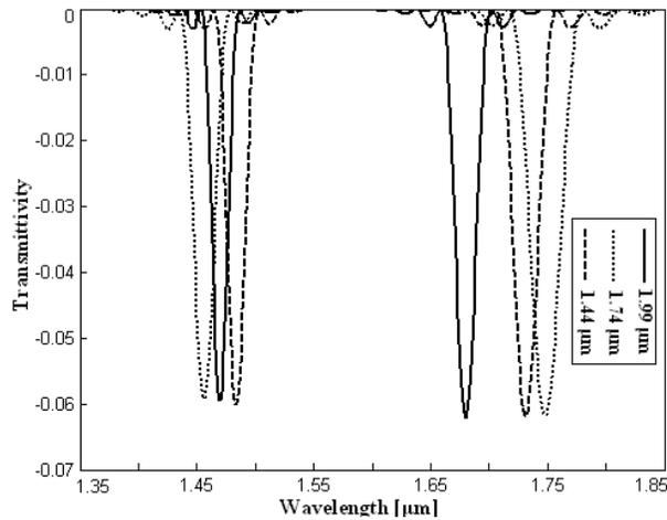
**Fig 6a:** Transmittivity vs wavelength of em wave for 15° oblique incidence for  $\text{Al}_{0.2}\text{Ga}_{0.8}\text{N}/\text{GaN}$  composition and constant well width but different barrier width
