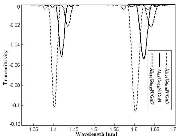
**Fig 2:** Transmittivity vs wavelength of em wave for normal incidence with constant layer dimensions and different material compositions
