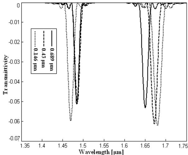
**Fig 6b:** Transmittivity vs wavelength of em wave for 15° oblique incidence for  $\text{Al}_{0.2}\text{Ga}_{0.8}\text{N}/\text{GaN}$  composition and constant barrier width but different well width
