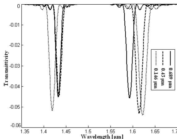
**Fig 3b:** Transmittivity vs wavelength of em wave for normal incidence for  $\text{Al}_{0.2}\text{Ga}_{0.8}\text{N}/\text{GaN}$  composition and constant barrier width but different well width
