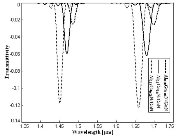
**Fig 5:** Transmittivity vs wavelength of em wave for 15° oblique incidence for constant layer dimensions and different material compositions
