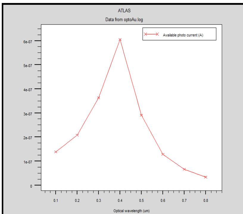
**Fig.9:** Photocurrent as a function of optical wavelength, for -0.5V.
