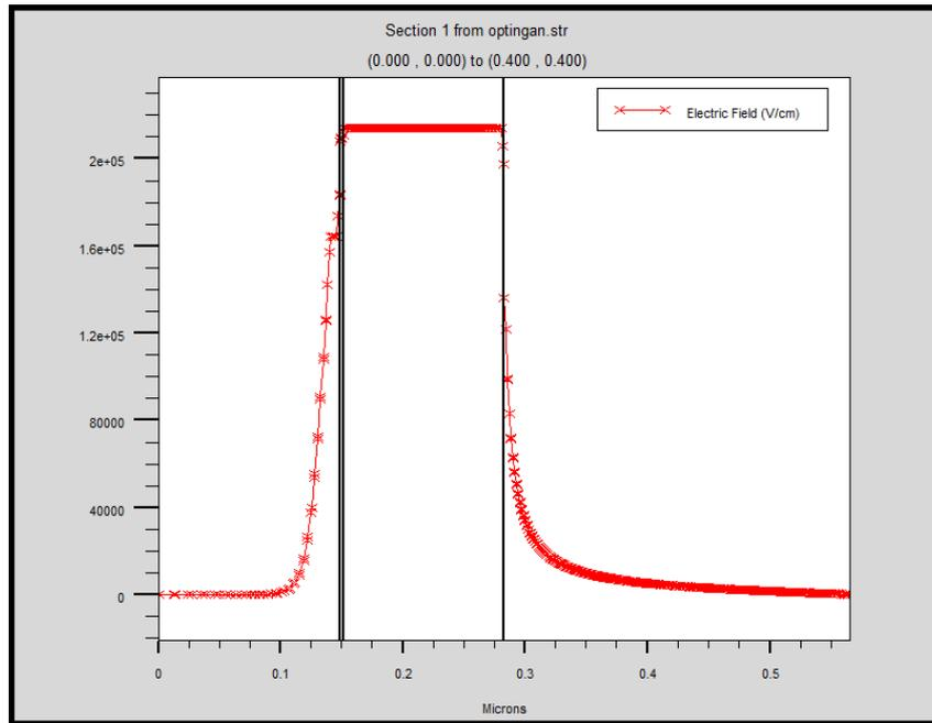
**Fig.4:** Simulated electric field profile in absence of external biasing.
