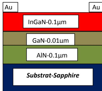
**Fig.2:** Structure of studied MSM UV photodetector with gold electrodes.
