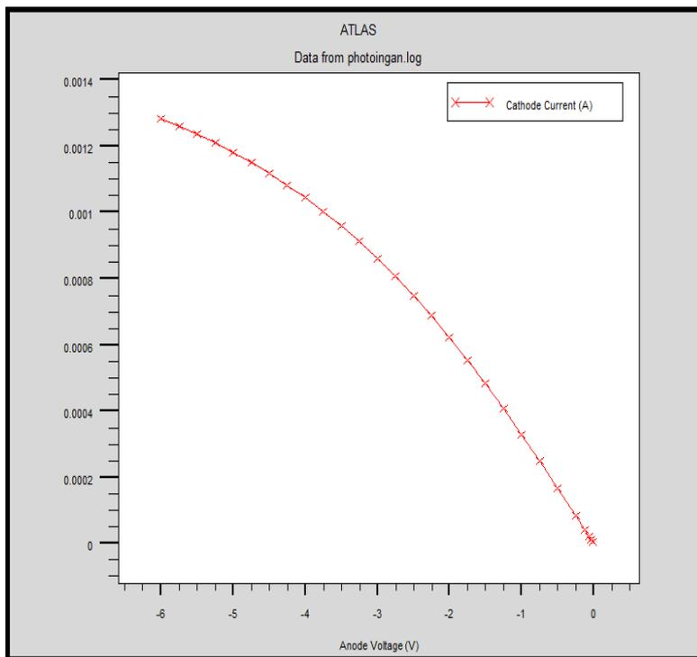
**Fig.8:** I-V curve in InGaN/GaN/AlN photodetector.
