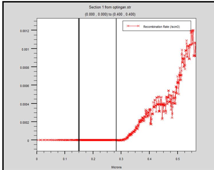
**Fig.6:** Recombination rate in the InGaN/GaN/AlN structure.
