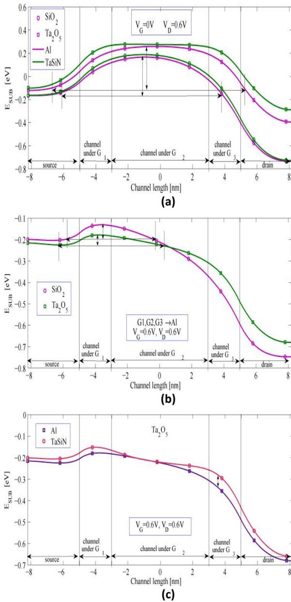
**Figure 4:** Potential profile along the middle of the Si channel with different dielectric layers for (a) Al and TaSiN-Al-TaSiN gates at  $V_G=0$  and  $V_D=600$  mV (b)  $Ta_2O_5$  and  $SiO_2$  layers with Al gates at  $V_G=600$  mV and (c) Al and TaSiN screen gates at  $V_G=600$  mV.
