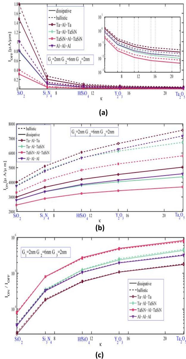
**Figure 2:** Plot of (a) on-current  $I_{ON}$  (b) off-current  $I_{OFF}$  and (c) on-off ratio  $I_{ON}/I_{OFF}$  (logarithmic scale) versus  $\kappa$ .
