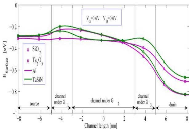
**Figure 6:** The surface potential along the channel of an Al gate device and a TaSiN-Al-TaSiN device for SiO<sub>2</sub> layer and Ta<sub>2</sub>O<sub>5</sub> layer.
