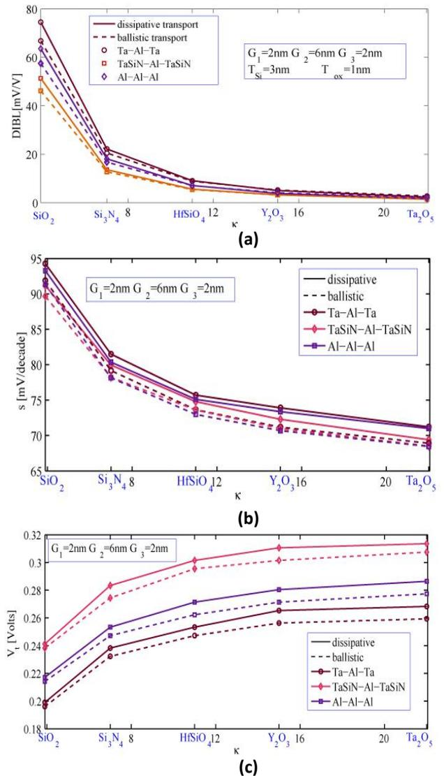
**Figure 5:** Plot of subthreshold parameters against dielectric constant. (a) DIBL (b) subthreshold swing  $S$  and (c) threshold voltage for different parallel connected gate materials.
