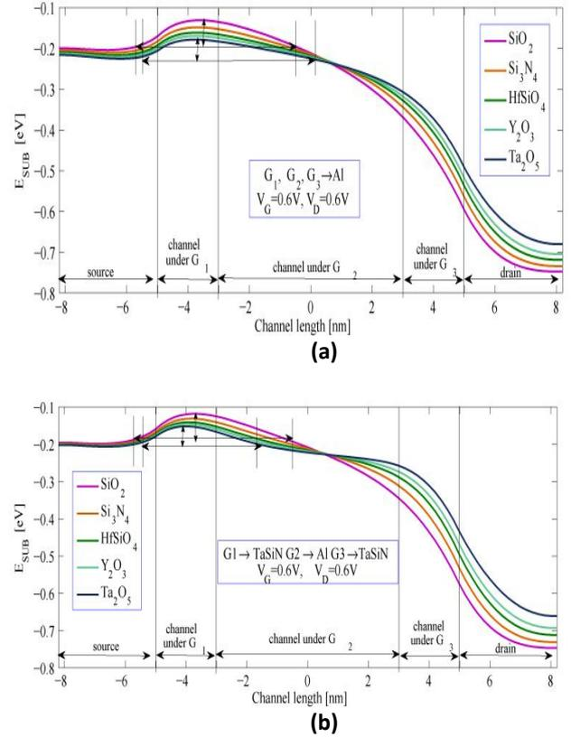
**Figure 3:** Potential profile along the middle of the Si channel with different high- $\kappa$  dielectric layers for a device (a) with Al and (b) with TaSiN-Al-TaSiN gates.
