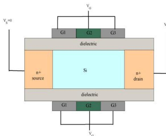
**Figure 1:** A Double Gate MOSFET with parallel connected metal contacts of different workfunctions forming the bottom and top gates.
