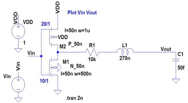
**Figure 3:** CMOS Driving RLC load
