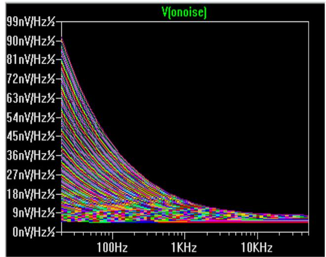
Figure 8: Output Noise Characteristics of CMOS Inverter without Skin Effect, at different temperatures
