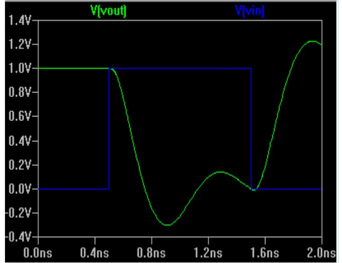
Figure 4: Delay Characteristics of CMOS Inverter without Skin Effect
