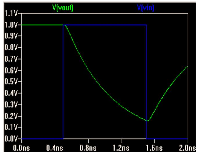
Figure 5: Delay Characteristics of CMOS Inverter with Skin Effect
