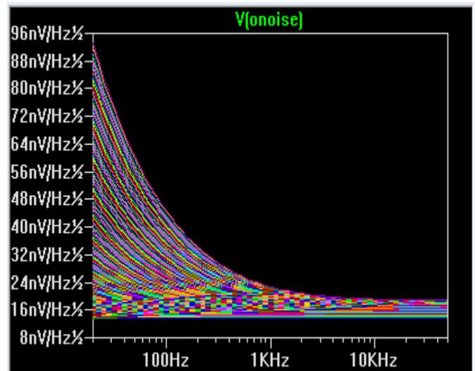
Figure 9: Output Noise Characteristics of CMOS Inverter with Skin Effect, at different temperatures.
