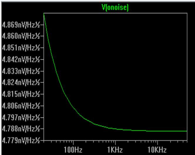
Figure 6: Output Noise Characteristics of CMOS Inverter without Skin Effect
