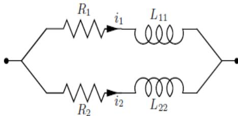
**Figure 2:** A circuit model with two different current paths with different Inductive properties
