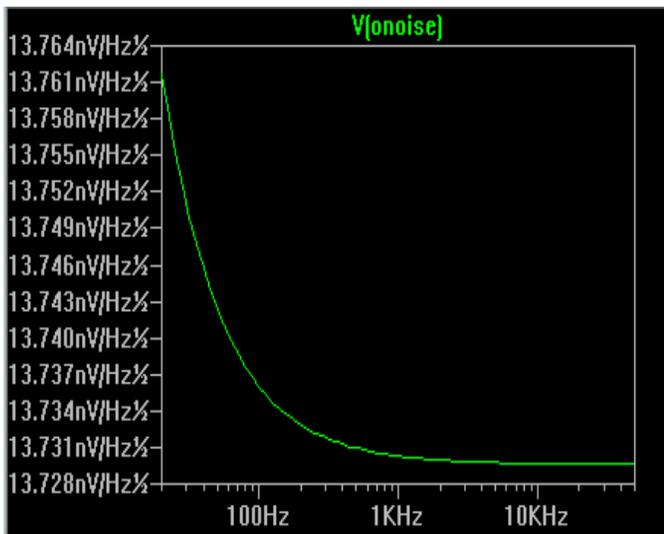
Figure 7: Output Noise Characteristics of CMOS Inverter with Skin Effect
