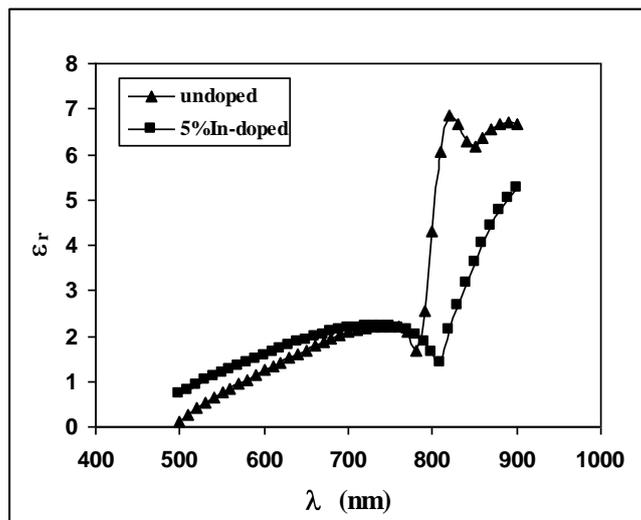
**Figure 5:** Variation of  $\epsilon_r$  with  $\lambda$  of undoped and 5%In-doped CdTe thin films.
