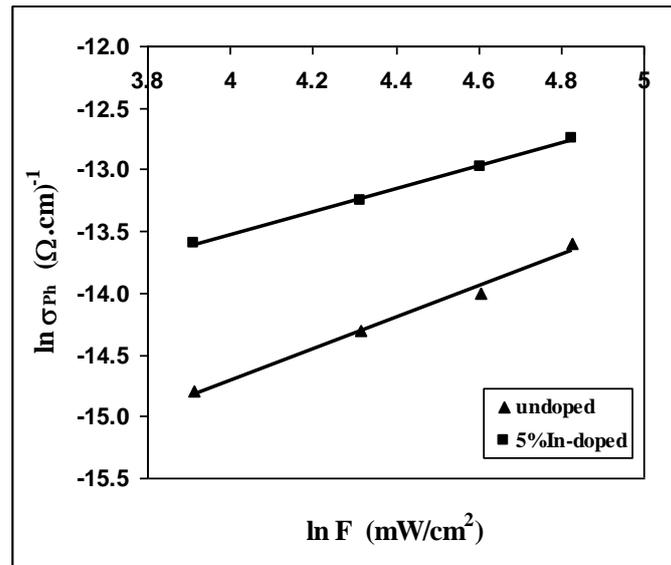
**Figure 7:** Variation of  $\ln(\sigma_{ph})$  vs.  $\ln(F)$  of undoped and 5% In-doped CdTe thin films.
