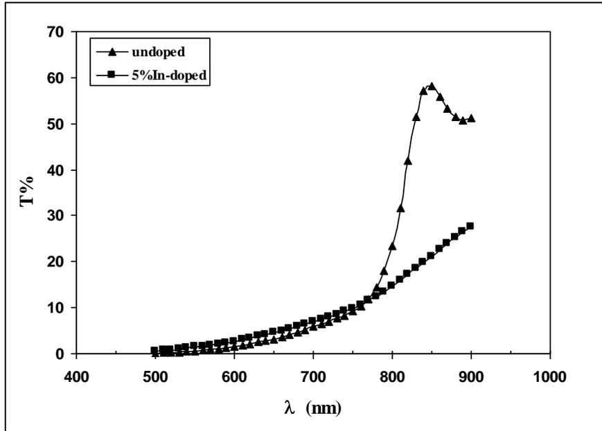
**Figure 1:** Transmittance spectra of undoped and 5%In-doped CdTe thin films.
