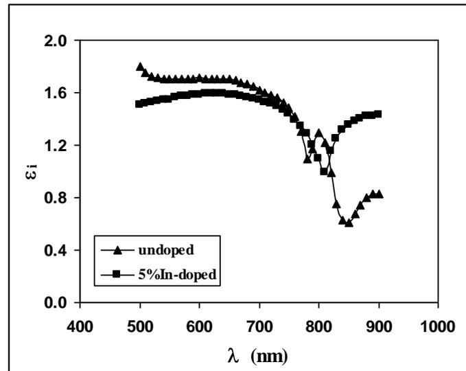
**Figure 6:** Variation of  $\epsilon_i$  with  $\lambda$  of undoped and 5%In-doped CdTe thin films.
