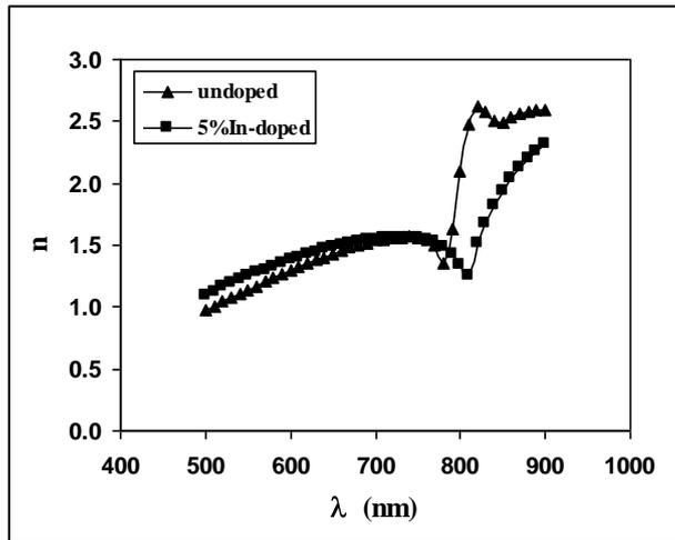
**Figure 3:** Variation of  $n$  with  $\lambda$  of undoped and 5%In-doped CdTe thin films.
