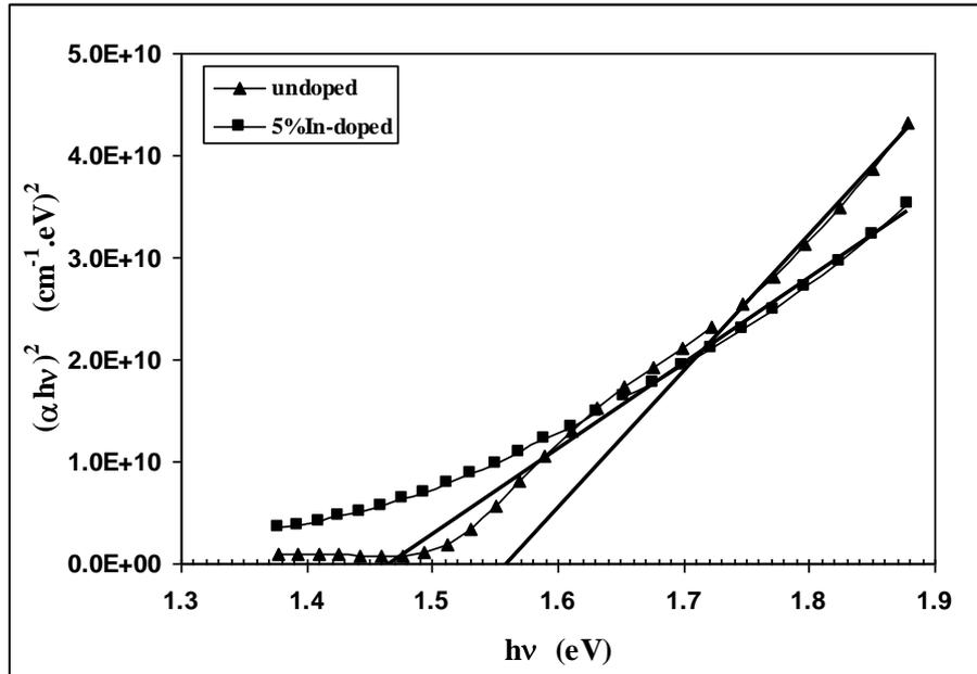
**Figure 2:**  $(\alpha hv)^2$  vs.  $h\nu$  of undoped and 5%In-doped CdTe thin films.
