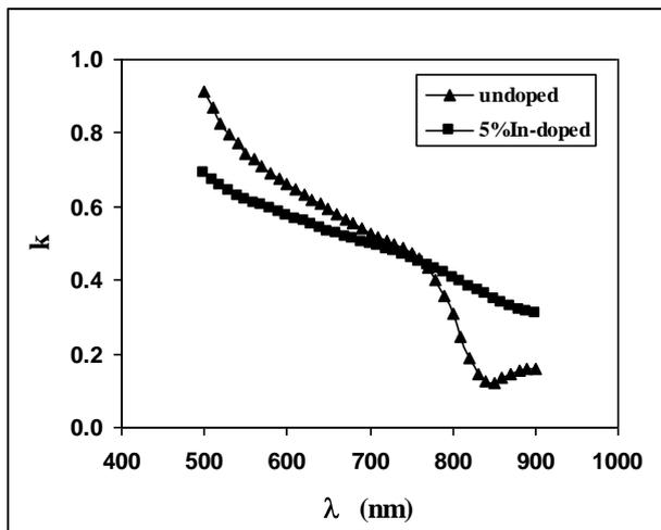
**Figure 4:** Variation of  $k$  with  $\lambda$  of undoped and 5%In-doped CdTe thin films.
