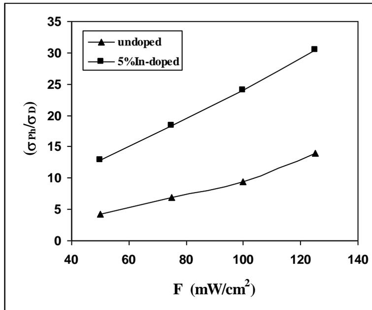
**Figure 8:** Variation of  $\sigma_{ph}/\sigma_D$  with  $F$  of undoped and 5% In-doped CdTe thin films.
