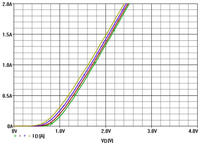
**Figure 5:** Forward characteristic at T= 25°C, 75°C, 125°C and 175°C (Yellow to Green)
