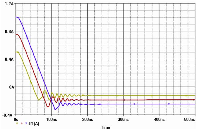
**Figure 8:** Turn-off Reverse Recovery Current of SiC Diodes for I<sub>1</sub> = 0.5A, 0.75 A and 1A (Yellow to Blue)
