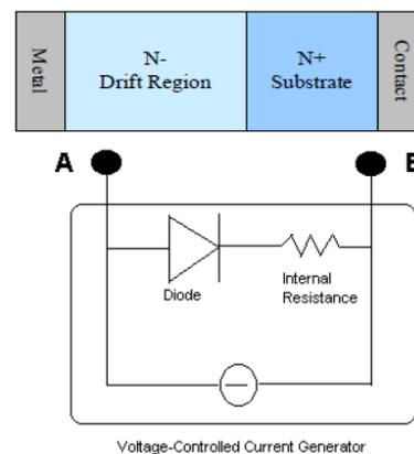
Figure 1: Electric Schottky diode Model
