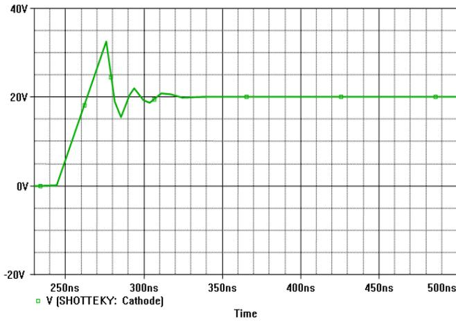
Figure 10: Forward recovery simulations of SiC Schottky
