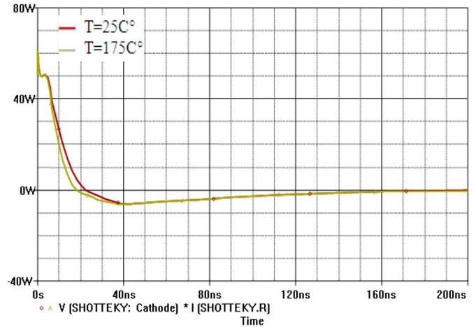
Figure 13: Power Loss during FET Turn-On for  $T=25^{\circ}\text{C}$  and  $T=175^{\circ}\text{C}$
