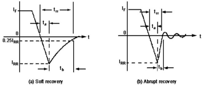
**Figure 2:** Reverse Recovery Current Characteristic
