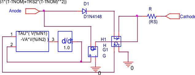
**Figure 3:** SPICE ABM static and dynamic SiC Schottky Diode Model
