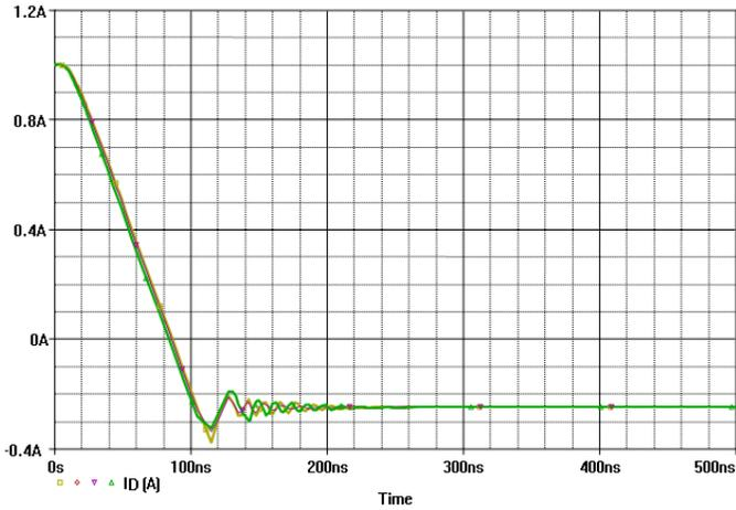
Figure 9: Turn-off transient for  $I_1 = 1$  A and  $T = 25$  °C, 75 °C, 125 °C and 175 °C.
