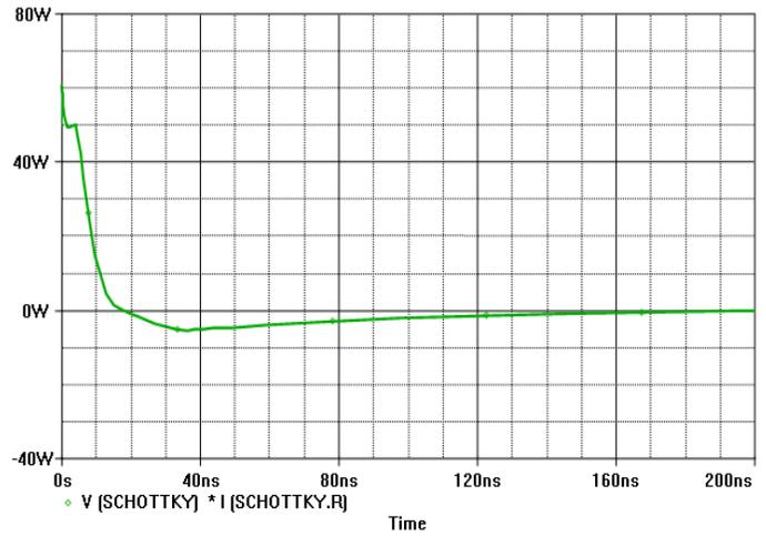
Figure 12: Power Loss during FET Turn-On
