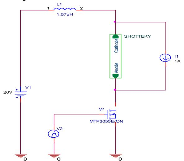
**Figure 6:** The test circuit used for simulation
