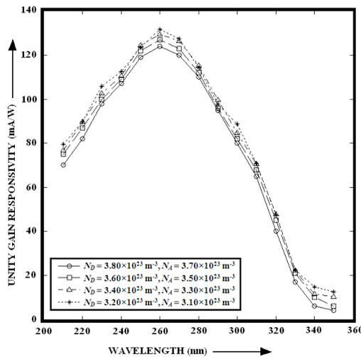
**Figure 5:** Variation of Unity Gain Spectral Responsivity with Wavelength in DDR 4H-SiC RAPDs due to optical illumination on the  $n^+$ -layer (FC structure).
