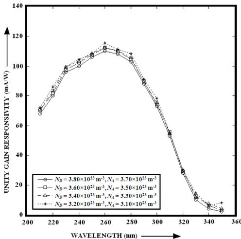
**Figure 6:** Variation of Unity Gain Spectral Responsivity with Wavelength in DDR 4H-SiC RAPDs due to optical illumination on the  $p^+$ -layer (TM structure).
