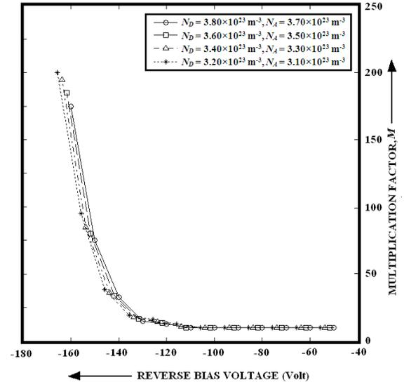
**Figure 4:** Variation of Multiplication Factor with Reverse Bias Voltage in DDR 4H-SiC RAPDs due to optical illumination on the  $p^+$ -layer (TM structure).
