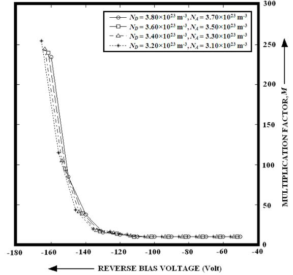
**Figure 3:** Variation of Multiplication Factor with Reverse Bias Voltage in DDR 4H-SiC RAPDs due to optical illumination on the  $n^+$ -layer (FC structure).
