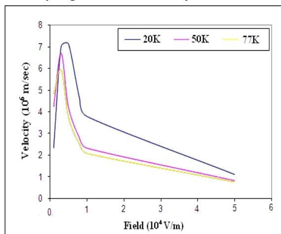
Fig.1: Velocity-field characteristics of CdSe at lattice temperatures of 20K, 50K and 77K.
