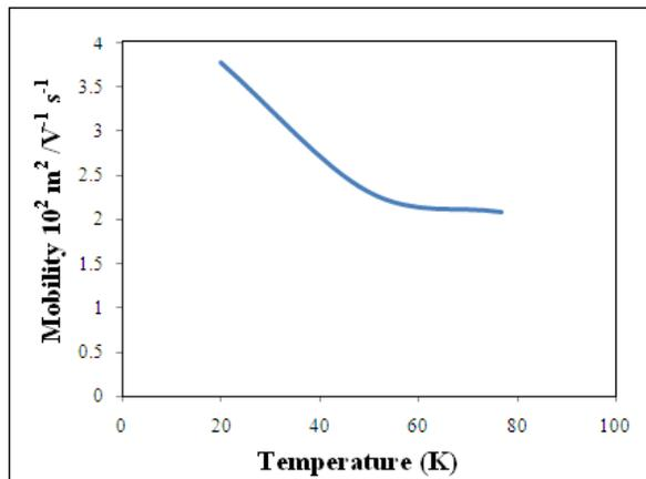
**Fig. 2:** Variation of electron drift mobility with lattice temperature.
