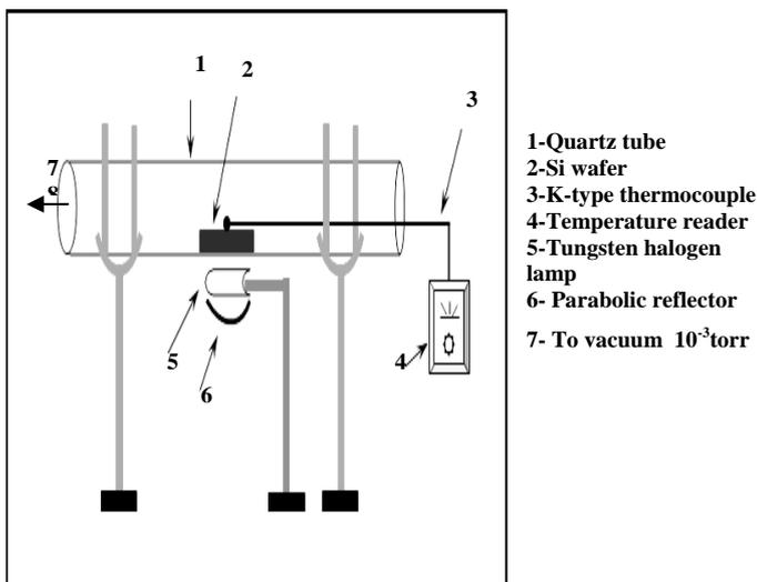
Figure 1: Rapid thermal diffusion system
