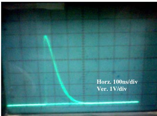
**Figure 6:** Laser pulse recorded by p-i-n photodetector
