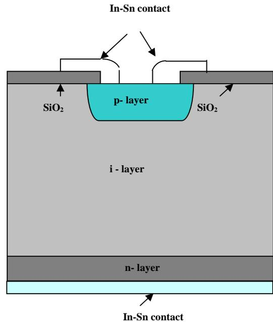
Figure 2: Cross sectional view of PIN silicon photodetector
