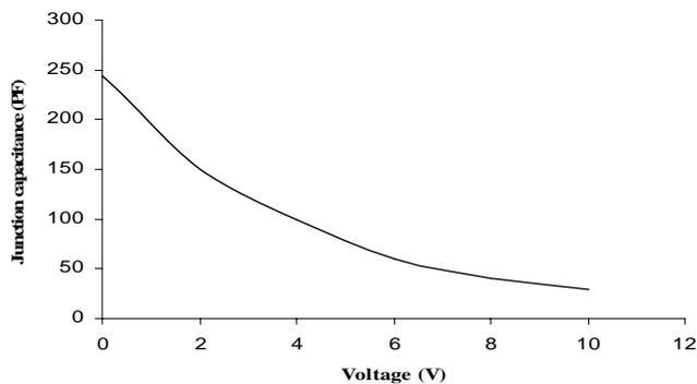
**Figure 4:** C-V characteristics of the photodiode
