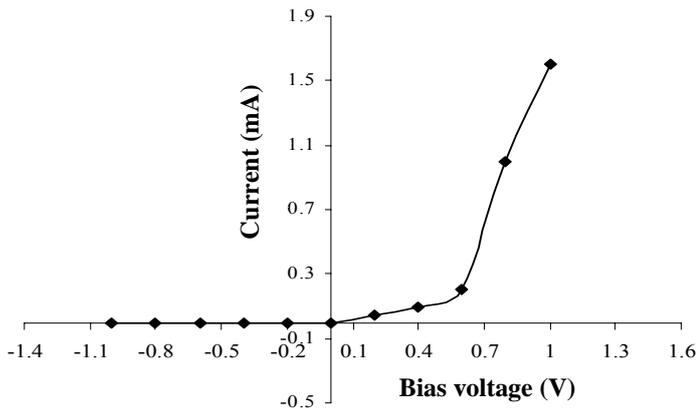
**Figure 3:** I-V characteristics of silicon p-i-n photodetector
