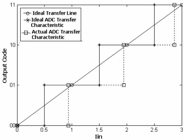
Figure 9. Ideal and simulated ADC characteristics
