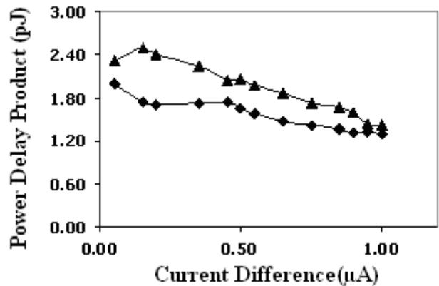
Figure 8. Power Delay Product versus current difference for Comparator I (▲) and II (◆)
