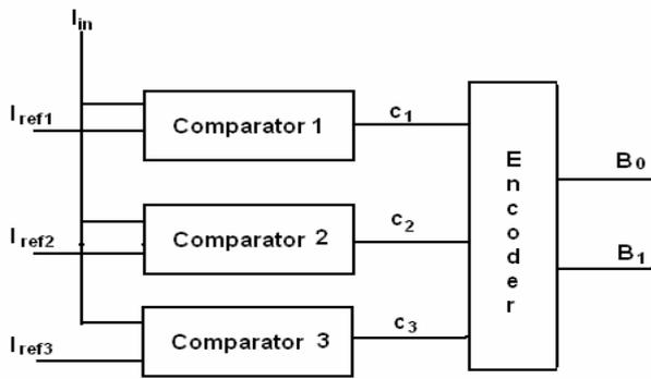
Figure 5. 2 bit Flash ADC
