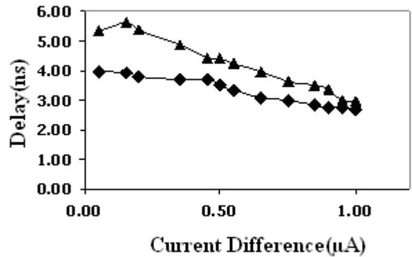
Figure 6. Delay versus current difference for Comparator I (▲) and II (◆)
