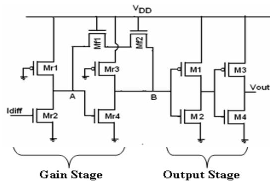
Figure 4. Gain and Output stage
