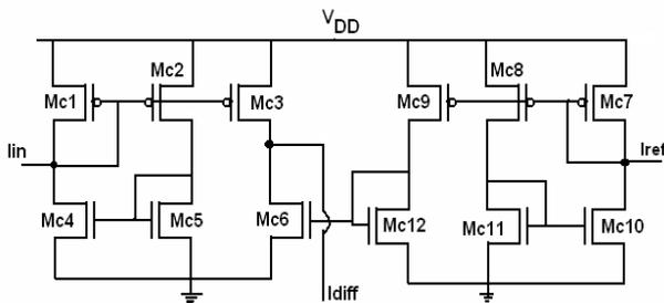
Figure 2. Current Difference stage
