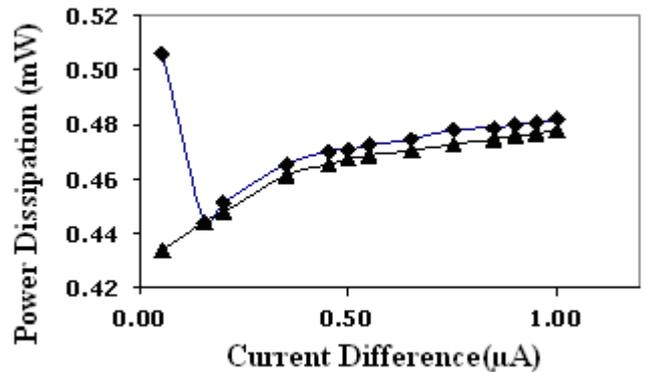
Figure 7. Power Dissipation versus current difference for Comparator I (▲) and II (◆)
