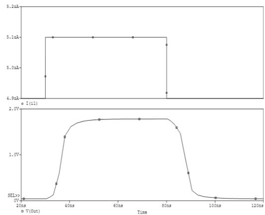
Figure 2 Simulation results for the proposed Current Comparator
