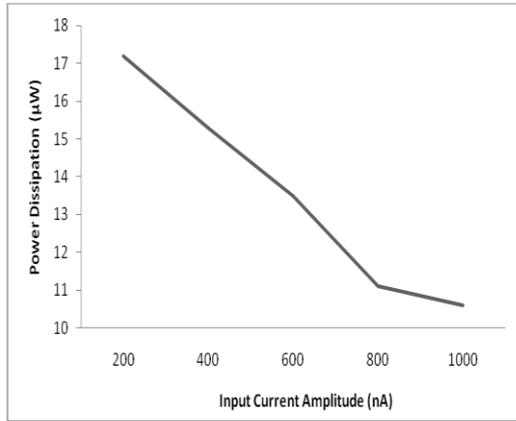
Figure 3. Variation in power dissipation with input current amplitudes
