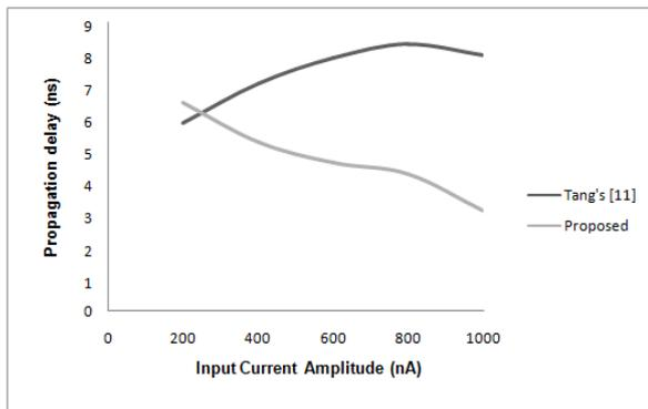
Figure 4. Variation of propagation delay with input current amplitudes
