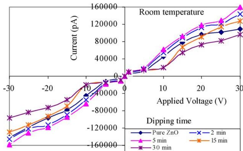
Fig. 1: I-V Characteristics of pure & CuO activated ZnO thick film
