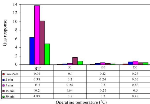
**Fig. 3:** Variaton of NH<sub>3</sub> gas response at different temperatures
