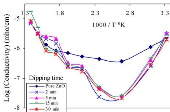
Fig. 2: Conductivity temperature profile of CuO activated ZnO films
